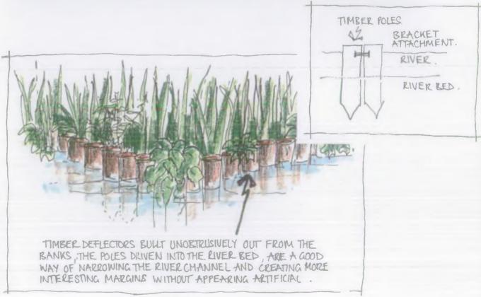
Timber deflectors can be used to mimic natural rafts of vegetation (above). Poles driven into the river bed can create spits of vegetation that can also form a narrowing of the channel.
