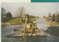
Hydraulic Excavator carrying out in channel weed control and cutting using herder cutter
