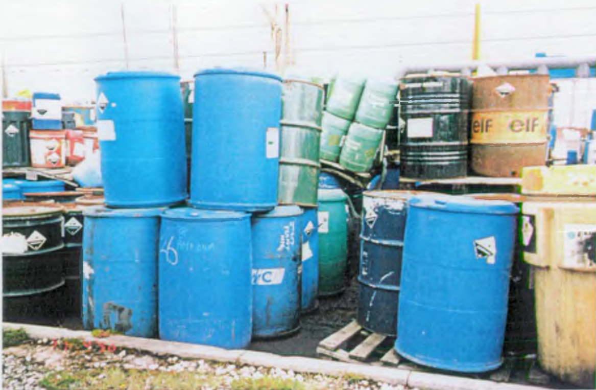
PHOTOGRAPH REF: SW/0169/005: DRUM HANDLING PLANT AREA 3 - POOR STACKING OF CONTAINERS
