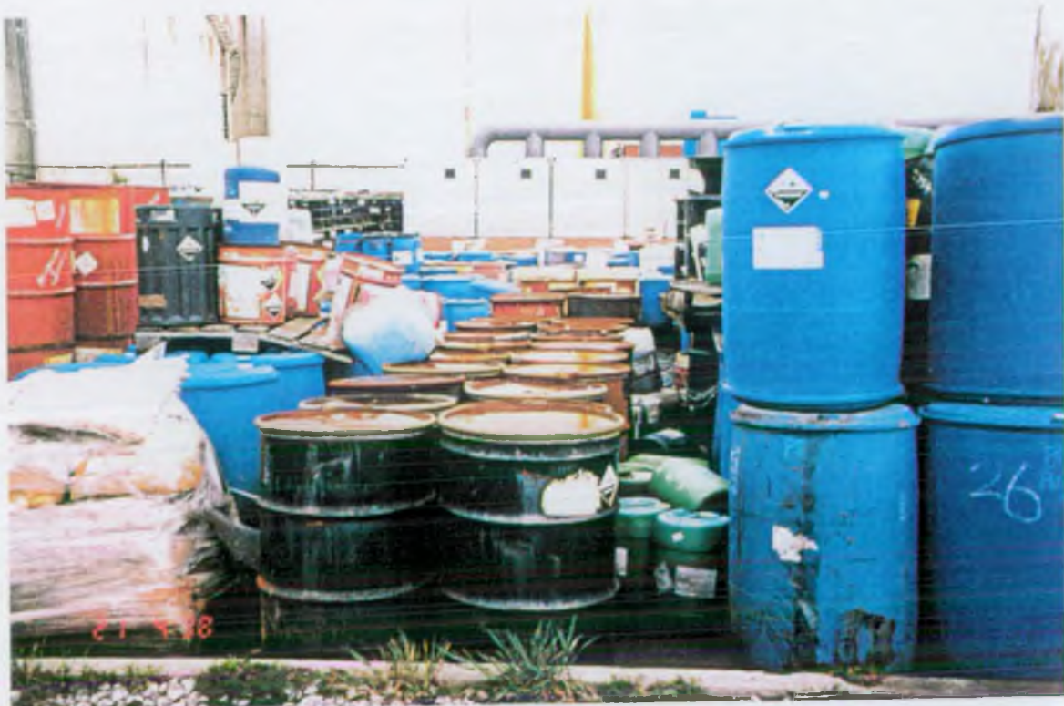
PHOTOGRAPH REF SW/0169/006: DRUM HANDLING PLANT AREA 3 - POOR STACKING OF CONTAINERS
