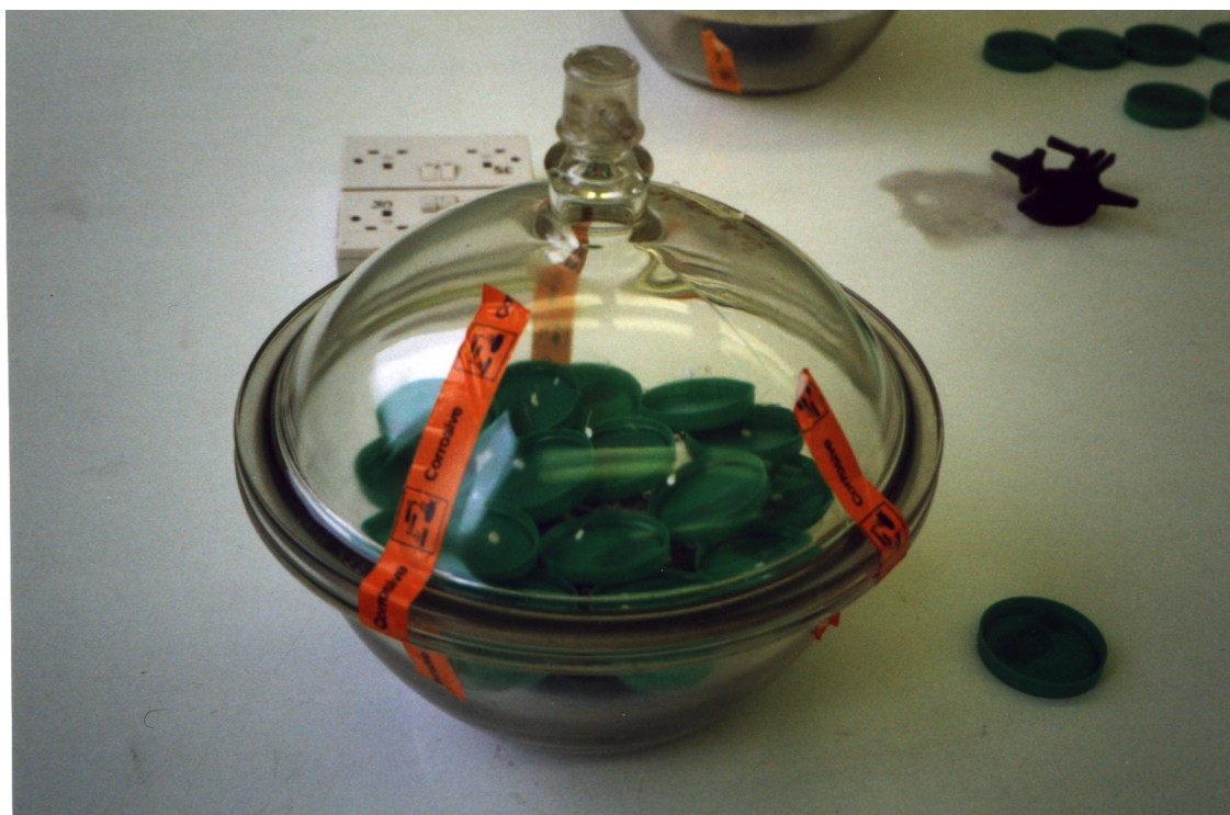
Figure 6.1 Desiccation of filter paper disks containing captured ammonia for continuous flow isotope ratio mass spectrometry.
