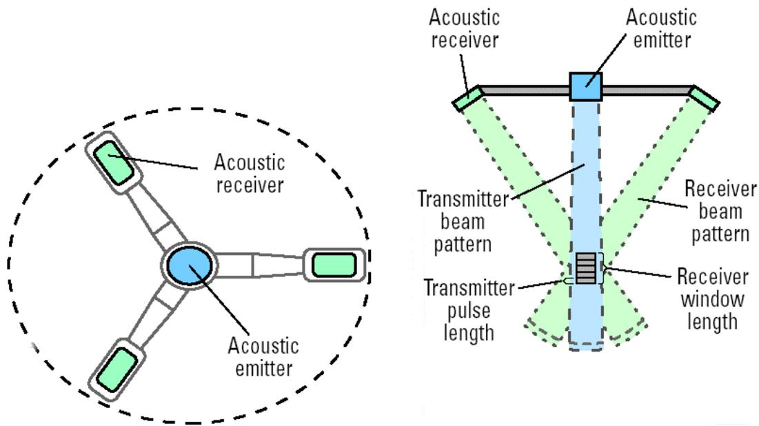
**Figure 2.2 Components of the Acoustic Doppler velocimeter showing acoustic emitter and receiver array (Wilson *et al.* 2001).**
