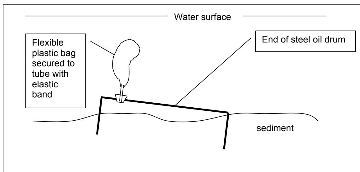
**Figure 4.1 Flexible bag seepage meter (after Lee 1977).**
