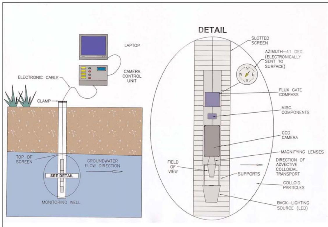
**Figure 2.3 The colloidal borescope (Newhouse and Hanson 2002).**
