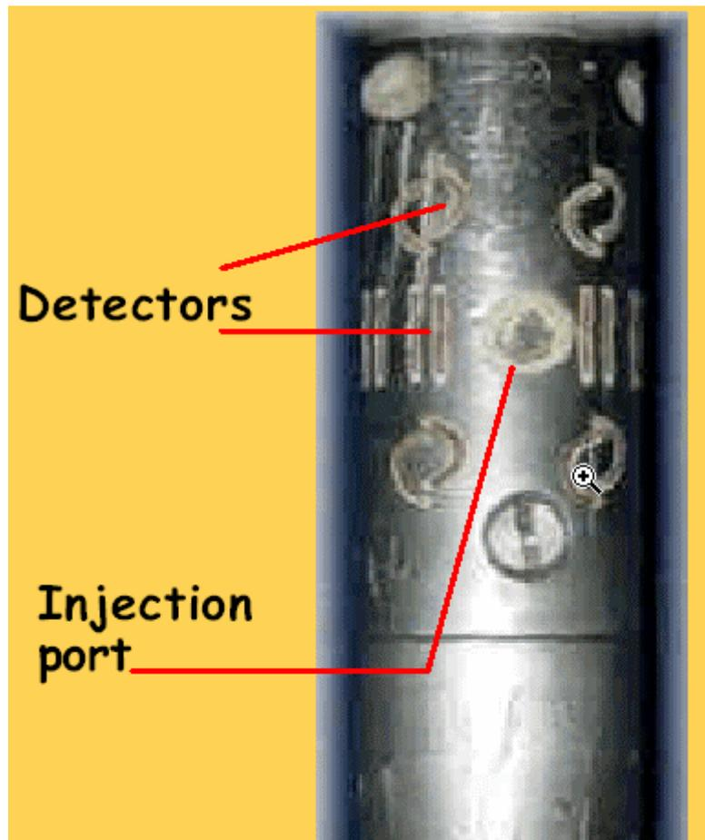
Figure 3.2 Tip of probe showing injection port and detectors (Labaky *et al.* 2002).
