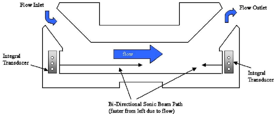
**Figure 4.6 Principle of the ultrasonic seepage meter (after Paulsen 2001a).**
