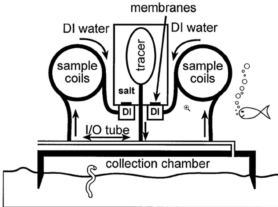
Figure 4.4 The benthic flux seepage meter of Tryon *et al.* (2001). DI = De-ionised (water).
