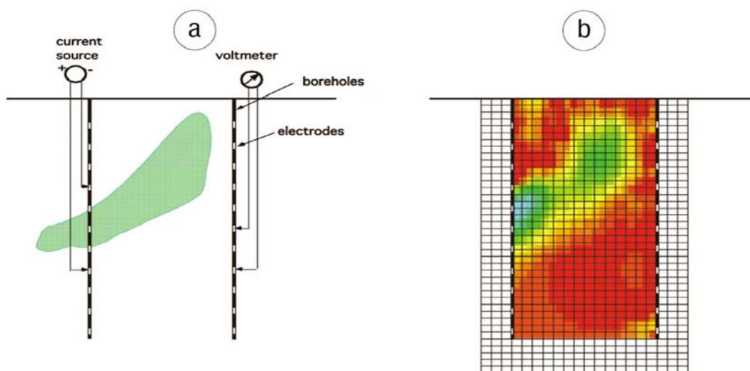
**Figure 5.1 Schematic representation of electrical resistance tomography showing the (a) arrangement of electrodes in a cross-hole array and (b) modelled image (Dailey *et al.* 2004).**
