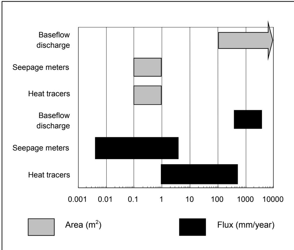
**Figure 1.1 Comparison of scales of measurement and rates of flux between various methods of determining recharge from surface waters, after Scanlon *et al.* (2002).**
