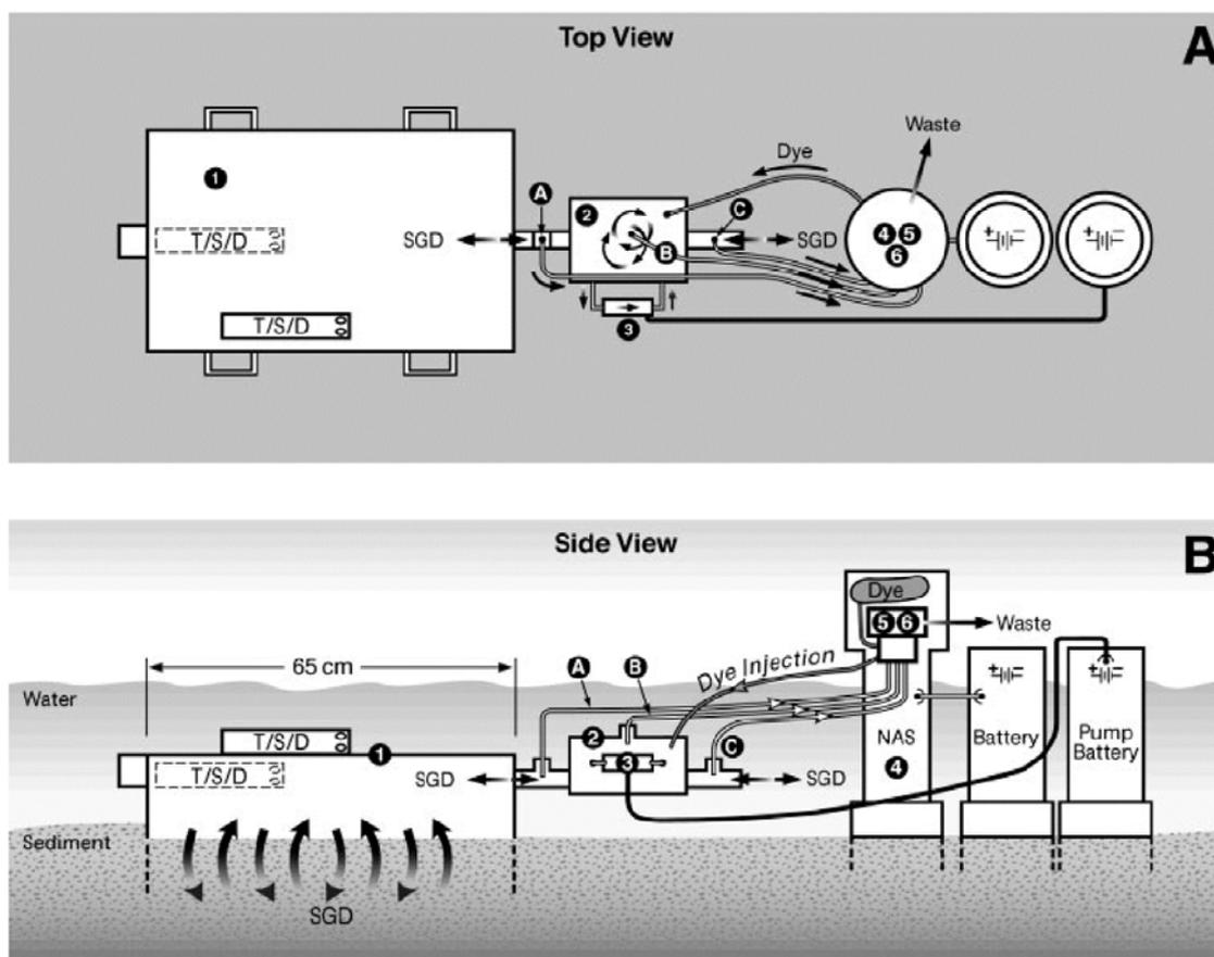
**Figure 4.3** The dye-dilution seepage flow meter (Sholkovitz *et al.* 2003). The seepage chamber (1) contains probes (T/S/D) to measure temperature, salinity and depth. Discharge (SGD) passes into the dye mixing chamber (2), where it mixed by a submersible pump (3) with dye injected from a chamber (4) that also houses a spectrometer to measure the concentration from sampling ports A, B and C.
