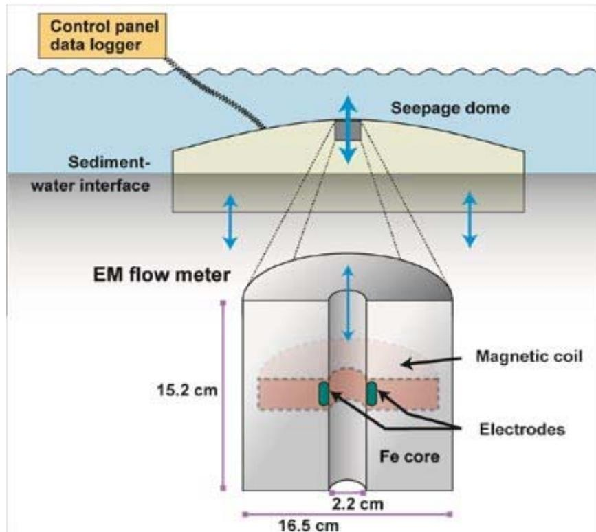
Figure 4.5 Electromagnetic (EM) seepage meter (Swarzenski *et al.* 2004).
