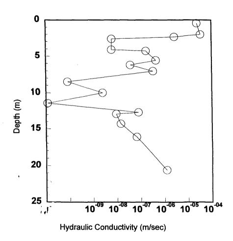
Figure 3.12 Hydraulic conductivity profile for Hall Farm
