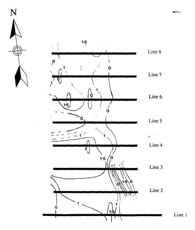
Figure 2.1 Contour plot of the depth to the base of the surface sand layer over the detailed apparent resistivity grid. Depths are in metres.
