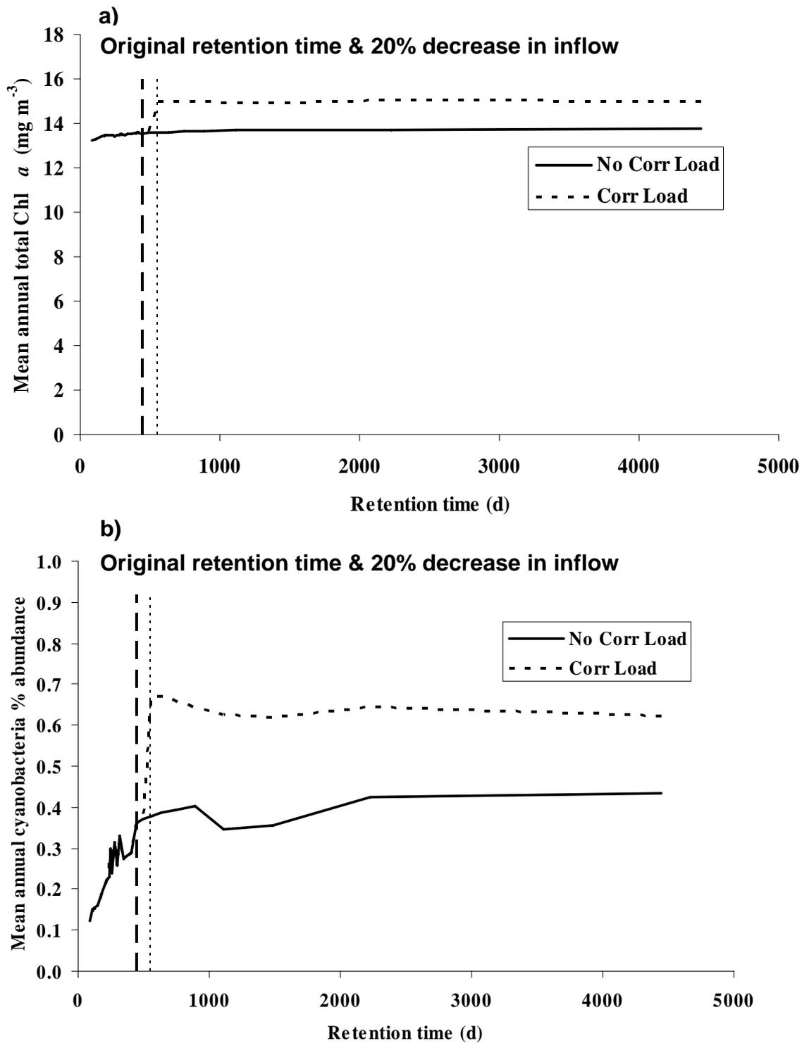
Fig. 20 Comparisons between the two methods of flow change for SE Reservoir with artificial mixing. a) Mean annual chlorophyll  $a$  biomass ( $\text{mg m}^{-3}$ ); b) Mean annual cyanobacteria percentage abundance. Note: No Corr Load describes the method where flow was simply multiplied and Corr Load the method that corrected the inflow concentrations.
