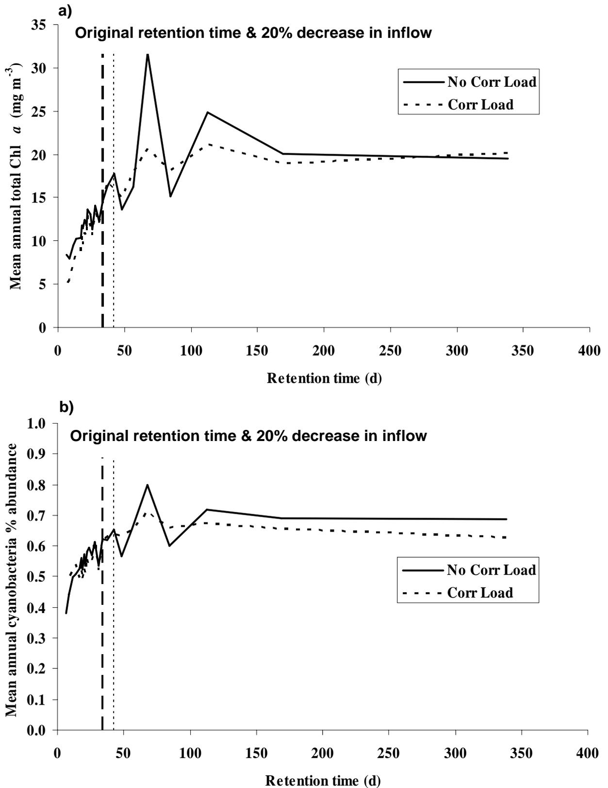
Fig. 12 Comparisons between the two methods of flow change for Blelham Tarn 1974. a) Mean annual chlorophyll *a* biomass ( $\text{mg m}^{-3}$ ); b) Mean annual cyanobacteria percentage abundance. Note: No Corr Load describes the method where flow was simply multiplied and Corr Load the method that corrected the inflow concentrations.
