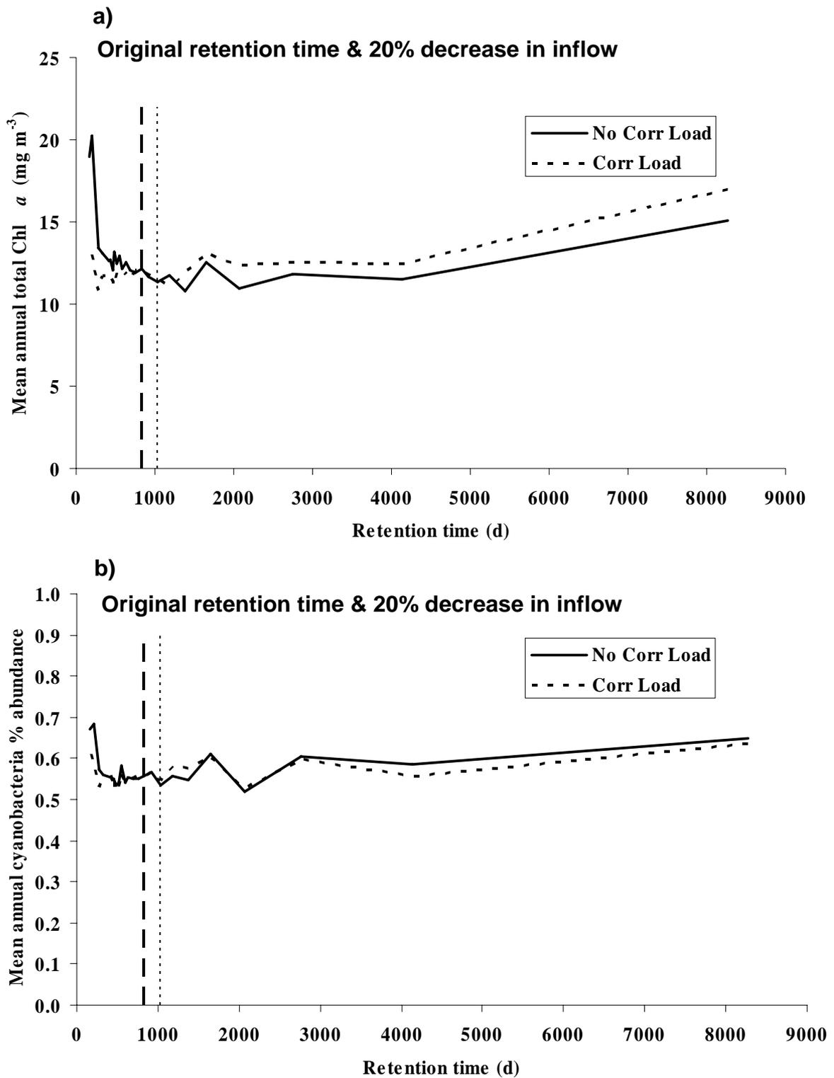
Fig. 14 Comparisons between the two methods of flow change for Rutland Water 1993. a) Mean annual chlorophyll *a* biomass ( $\text{mg m}^{-3}$ ); b) Mean annual cyanobacteria percentage abundance. Note: No Corr Load describes the method where flow was simply multiplied and Corr Load the method that corrected the inflow concentrations.
