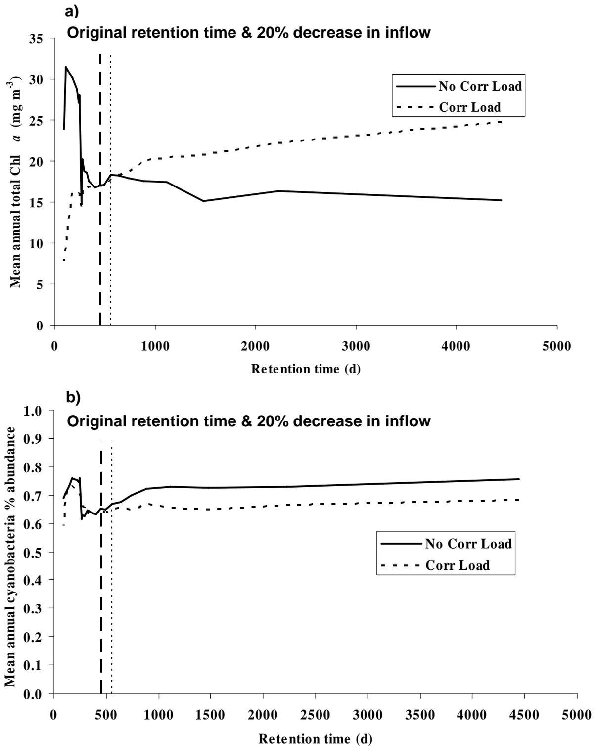
Fig. 18 Comparisons between the two methods of flow change for SE Reservoir. a) Mean annual chlorophyll *a* biomass ( $\text{mg m}^{-3}$ ); b) Mean annual cyanobacteria percentage abundance. Note: No Corr Load describes the method where flow was simply multiplied and Corr Load the method that corrected the inflow concentrations.
