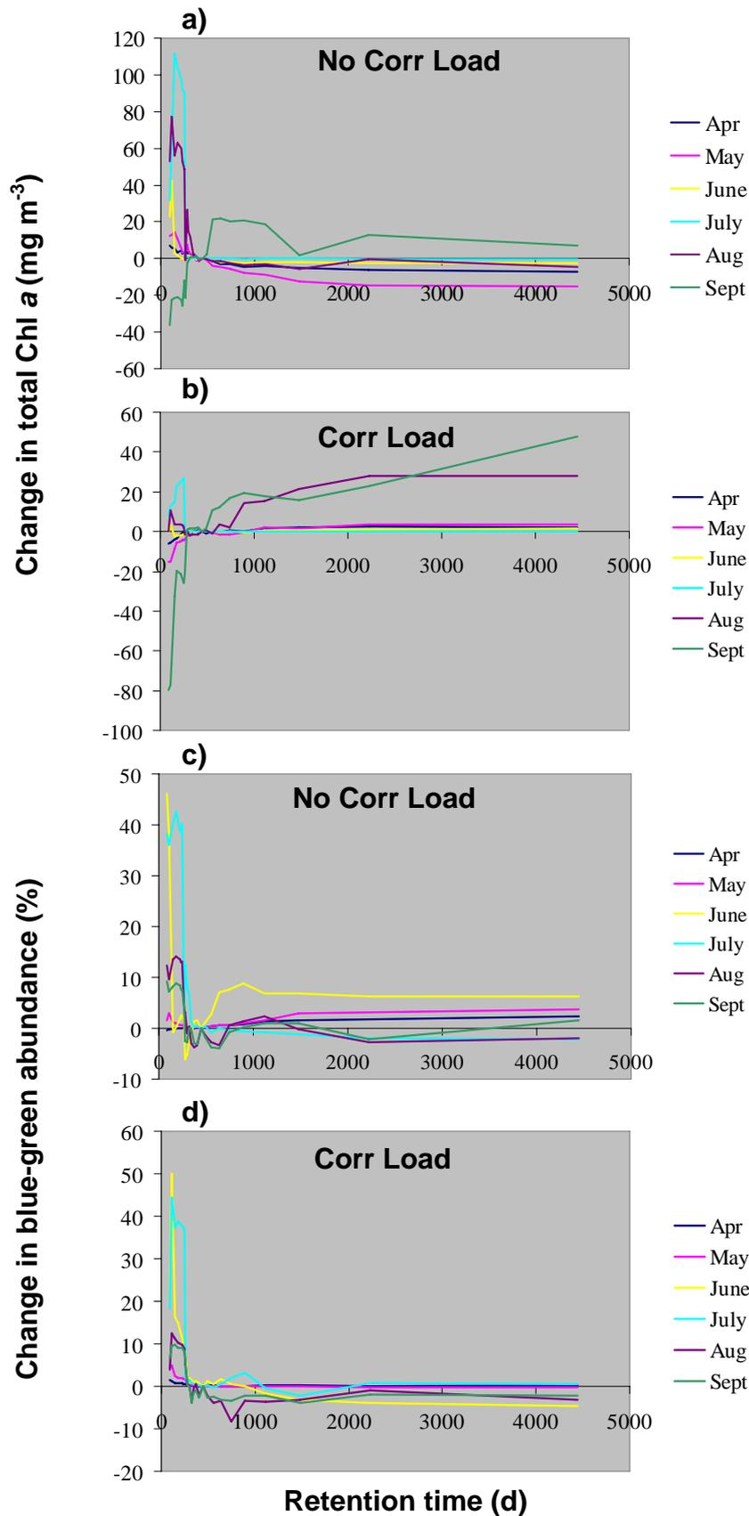
Fig. 19 Comparisons for SE Reservoir. a & b) Absolute change in monthly mean chlorophyll a biomass (mg m<sup>-3</sup>) and; c & d) monthly cyanobacteria percentage abundance for April-September for both flow methods.
