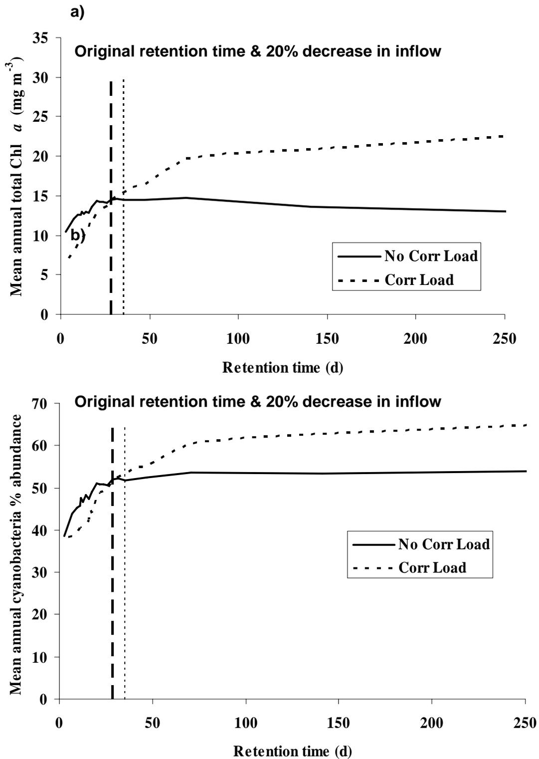
Fig. 6 Comparisons between the two methods of flow change for Bassenthwaite Lake 1996. a) Mean annual chlorophyll *a* biomass ( $\text{mg m}^{-3}$ ); b) Mean annual cyanobacteria percentage abundance. Note: No Corr Load describes the method where flow was simply multiplied and Corr Load the method that corrected the inflow concentrations.
