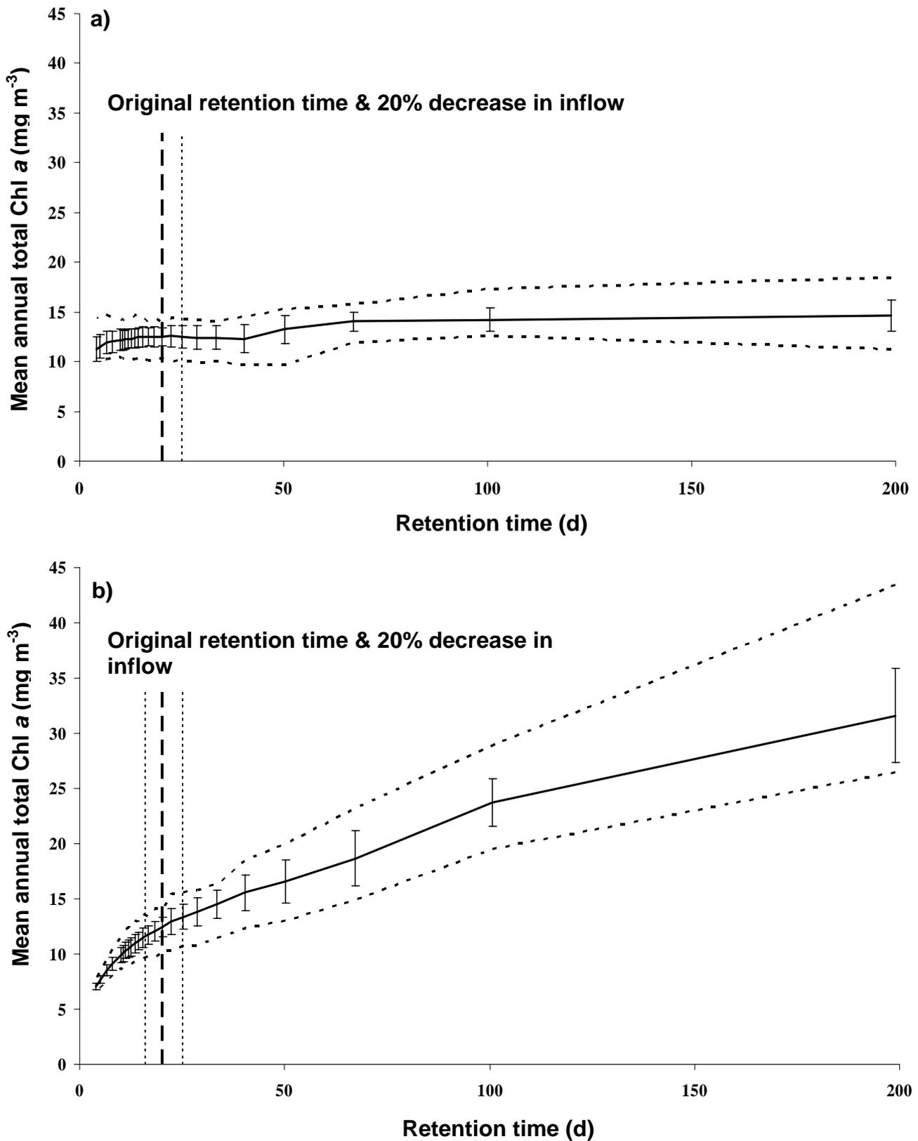
Fig. 10 Comparisons of mean annual chlorophyll a biomass ( $\text{mg m}^{-3}$ ) between the two methods of flow change for Bassenthwaite Lake 20 year run. a) No Corr Load; b) Corr Load. Dotted lines indicate maximum and minimum values and bars show 1 standard deviation.
