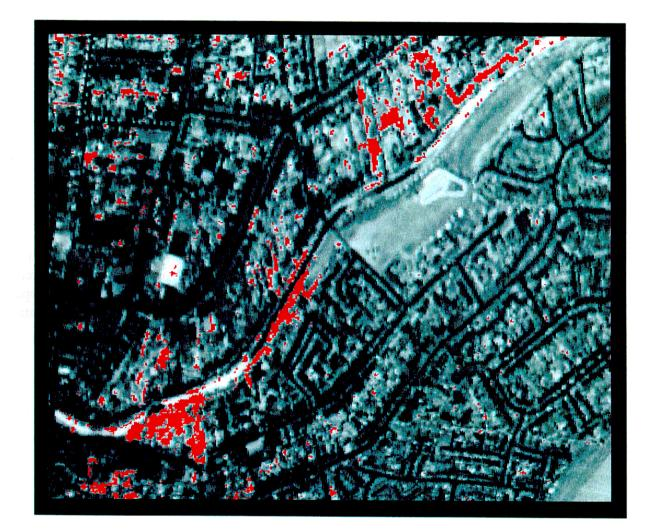
Figure 17: CASI image of March, Cambridgeshire. The image shows the near infra-red band, with areas of healthy vegetation highlighted in red.
