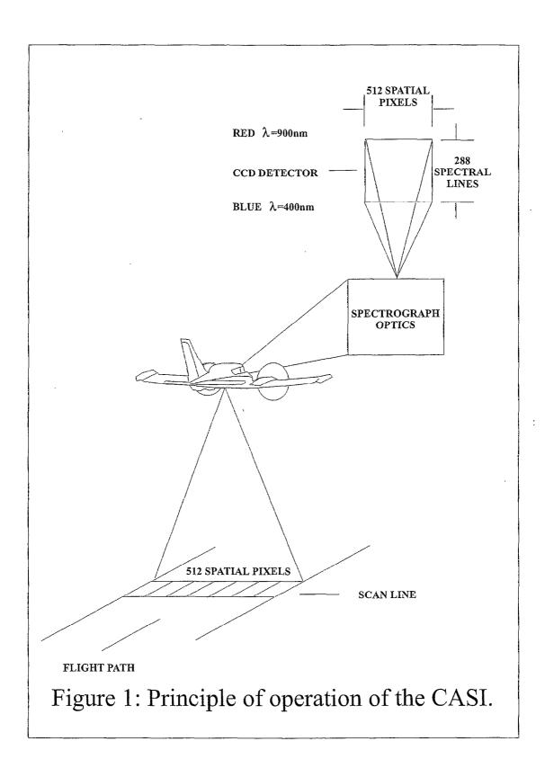
The CASI uses a Charge Coupled Device (CCD) detector to produce hyperspectral imagery which can comprise up to 288 spectral bands (wavebands), covering the electromagnetic spectrum from 430 nm (visible blue light) to 900 nm (Near Infra-red).
