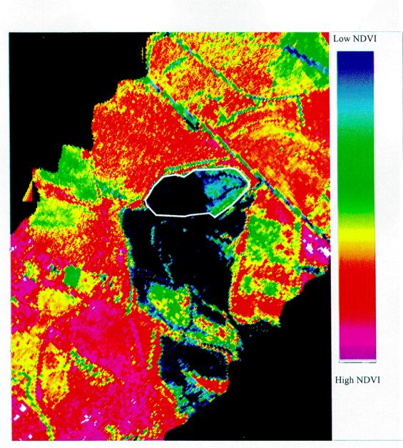
Figure 22 :NDVI image of Tatchells landfill site, colour coded to pick out high biomass areas in pink/red and low biomass areas in blue.
