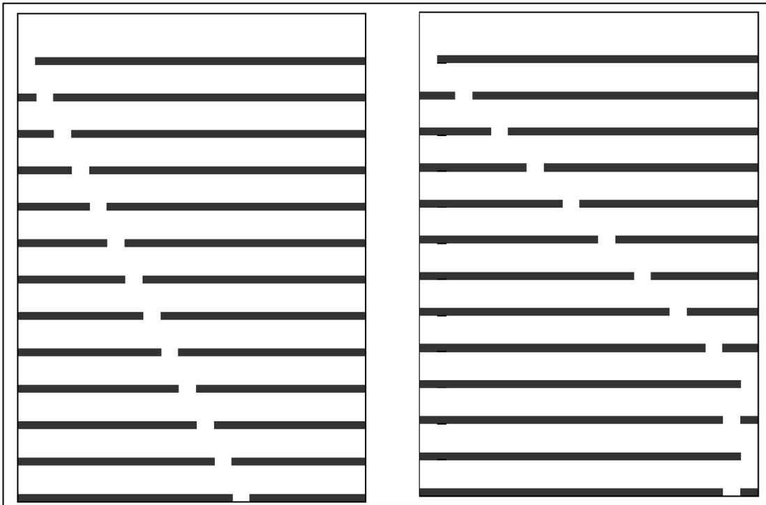
**Figure 3.4** Oblique channel with increasing stagger and constant slot width
