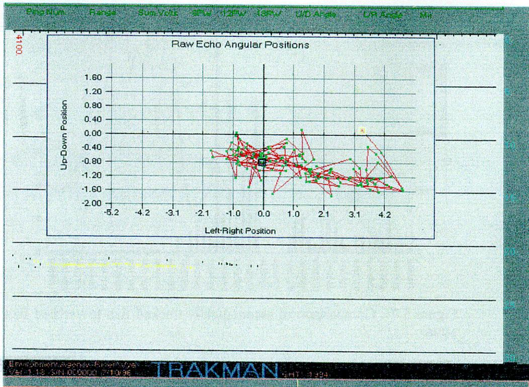
Figure 5.6: Example of a single fish trace that was broken up into several fish by the automated tracking software.
