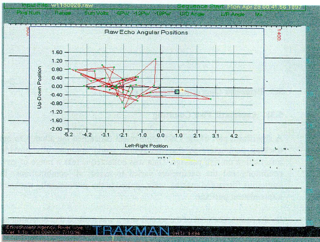
Figure 5.5: Downstream moving target with 2 stray final echoes causing the appearance of net upstream movement.
