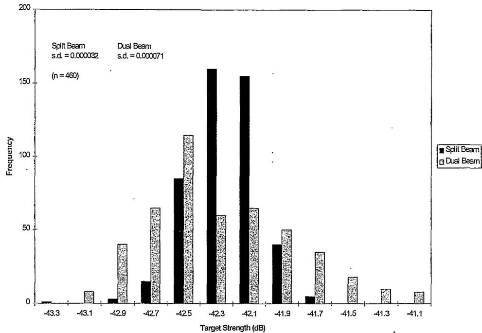
Figure 2.3: Target strength measurements of a tungsten carbide sphere using the dual-beam and split-beam techniques (Traynor and Ehrenberg, 1990).
