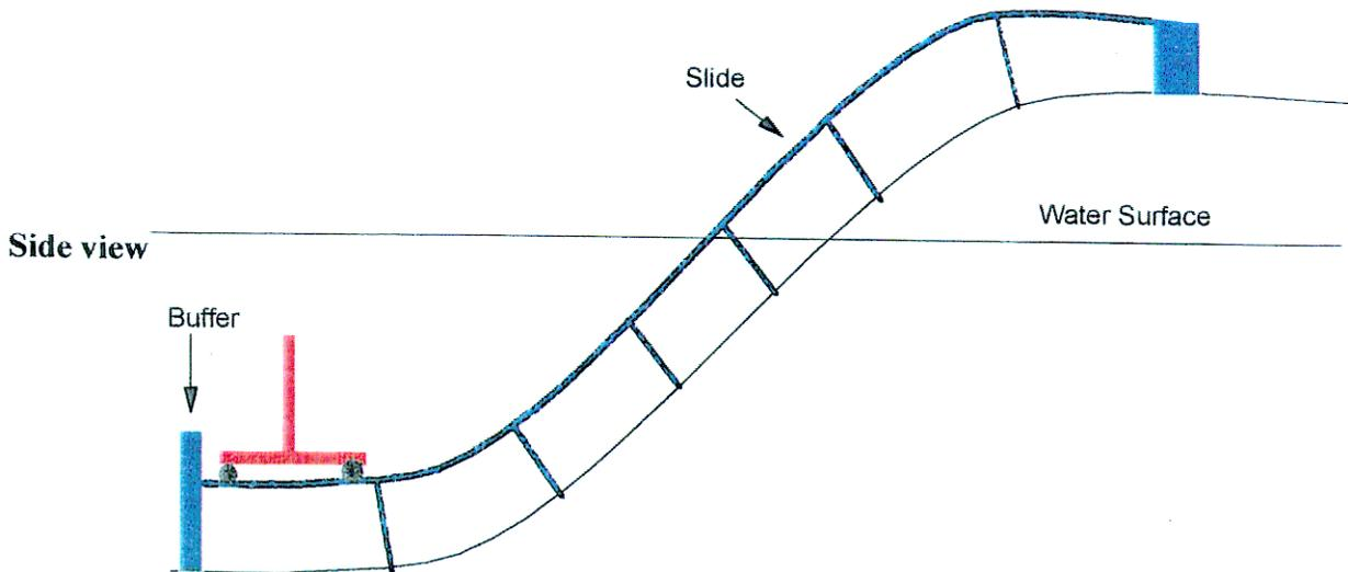
**Figure 3.3** Diagram of the "slide and trolley" mount designed for the Wye.
