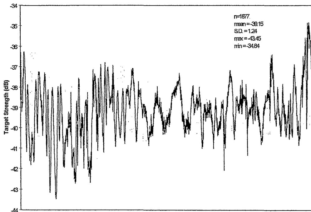
Figure 5.3: Ping to ping target strength variation during a standard target test.
