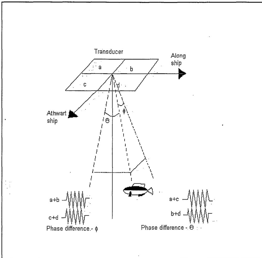
Figure 2.2 Diagram showing the principles of a split-beam echosounder from the perspective of a vertically aimed transducer.
