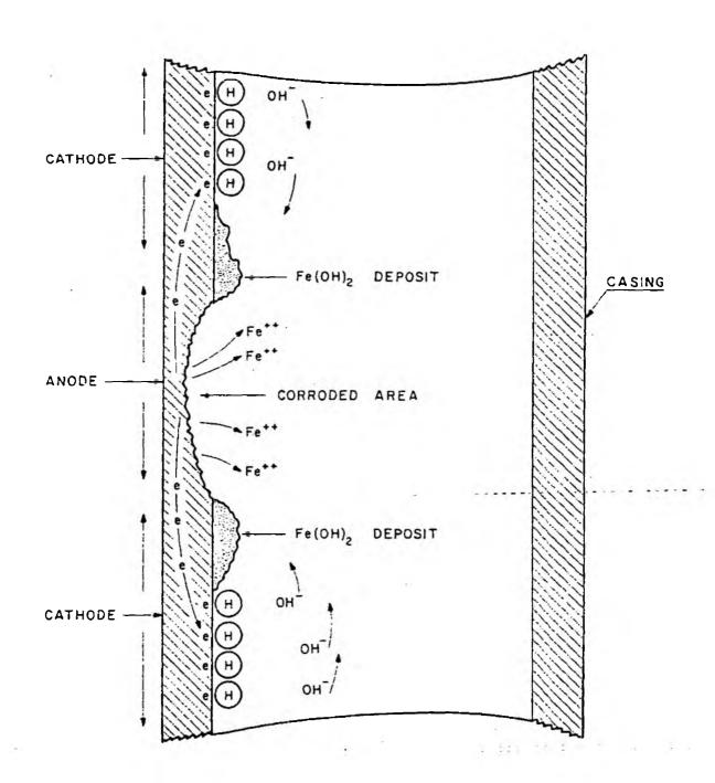
Electrolytic Corrosion Process
