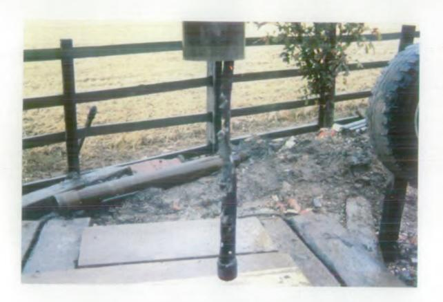
2" casing reduced to typical Lacework structure by acid attack. Note: thicker casing collar (at bottom of casing) resists attack.
