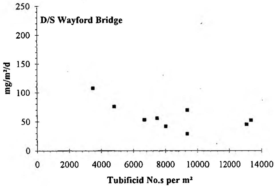
**Figure 4.3** The relationship between the ammonium release rate (mg/m<sup>2</sup>/d) and the number of tubificids in the cores (No. per m<sup>2</sup>)
