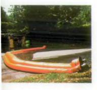
The first method of dealing with oil pollution on a river is likely to be the use of an absorbant boom. This has the capacity to absorb oil but repel water. The boom is deployed across the river and secured at each end using stakes.
