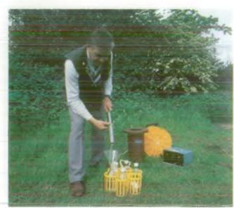
Taking a sample of groundwater from an observation borehole.
