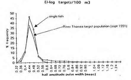
3. Frequency distribution of half-amplitude pulse widths for a fish population in the River Thames near Didcot (black squares) compared with a single perch of 120 mm length (side aspect) (empty squares).
