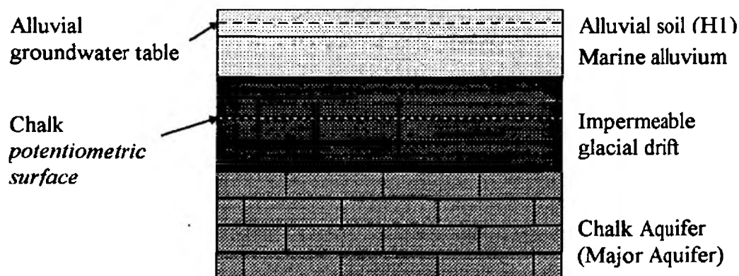
Figure 5.1 Diagrammatic cross section of the possible misrepresentation of the groundwater vulnerability of some confined aquifers.
