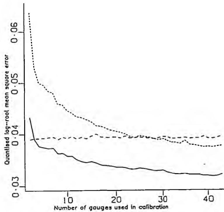
The effect of number of gauges on rainfall estimation accuracy. Results averaged over 13 events. Continuous line: calibrated radar; short dashes: raingauge-only; long dashes: uncalibrated radar.
