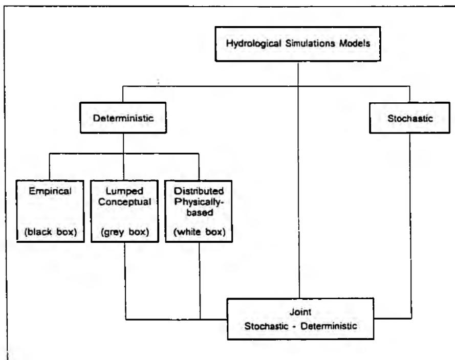
Figure 3.9 Classification of hydrological models according to process description.
