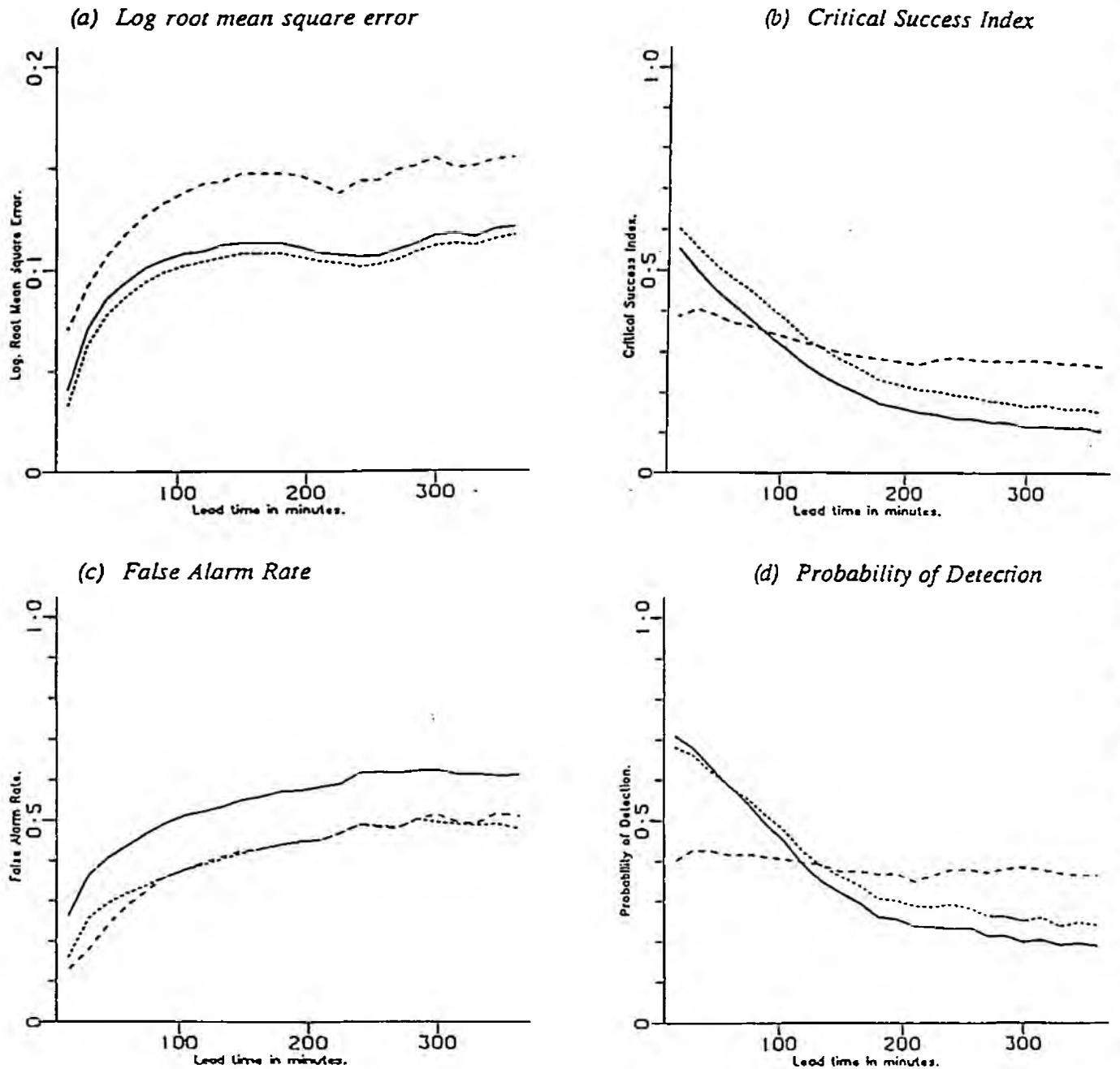
Rainfall accumulation forecast error statistics, averaged over 14 storm events, for different lead times: radar data as truth (continuous line: 2 km local forecast; short dashes: 5 km local forecast; long dashes: Frontiers forecast)
