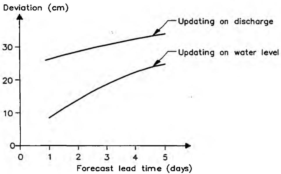
Figure 3.11 Comparison of forecast accuracy by hydraulic routing using updating on water levels and discharge, from DHI 1994.
