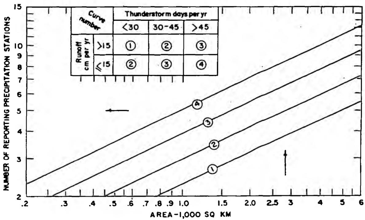
Figure 3.6 Raingauge network design curves for forecasting applications, from Nemeč, 1986.
