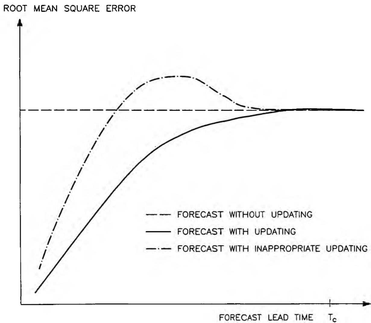
Figure 2.2 General behaviour of forecasting error as a function of lead time.
