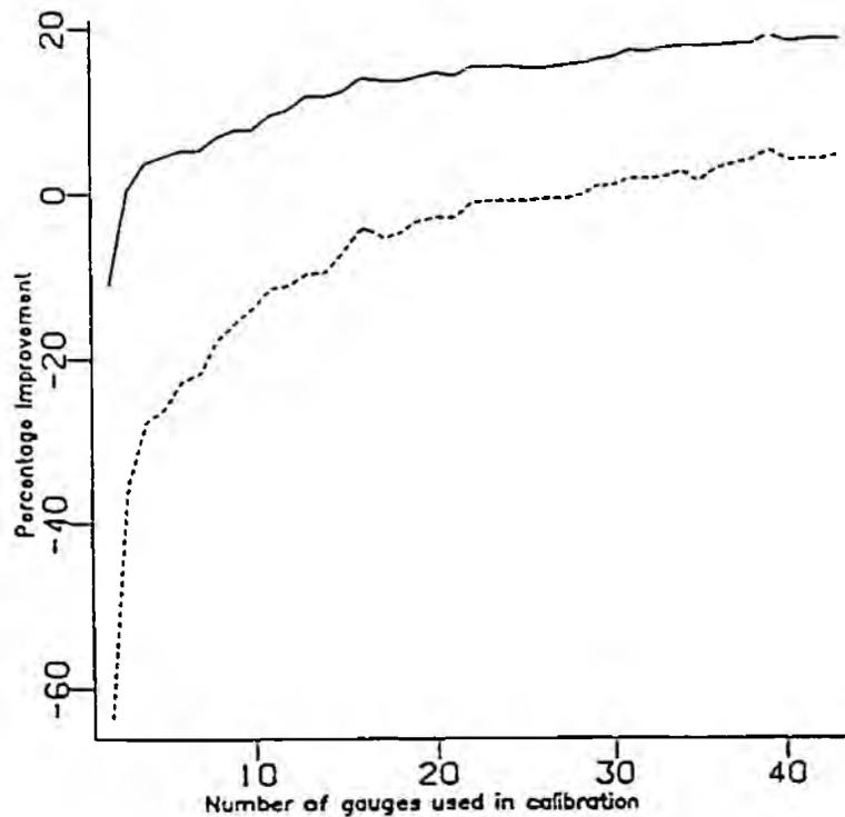
Percentage improvement in performance of raingauge-only (dashed line) and calibrated radar (continuous line) estimates of rainfall, relative to uncalibrated radar, as a function of number of raingauges in network. Results averaged over 13 events.
