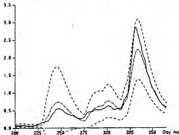
Simulated streamflows with confidence limits assuming: (a) only uncertainty on precipitation input ( $\sigma_p = 60\%$ ,  $\sigma_{K1} = 0$ ,  $\sigma_{COF} = 0$ ); (b) uncertainty on model parameters ( $\sigma_p = 0$ ,  $\sigma_{K1} = 15\%$ ,  $\sigma_{COF} = 5\%$ ); (c) uncertainty on both precipitation input and model parameters ( $\sigma_p = 60\%$ ,  $\sigma_{K1} = 15\%$ ,  $\sigma_{COF} = 5\%$ ).
