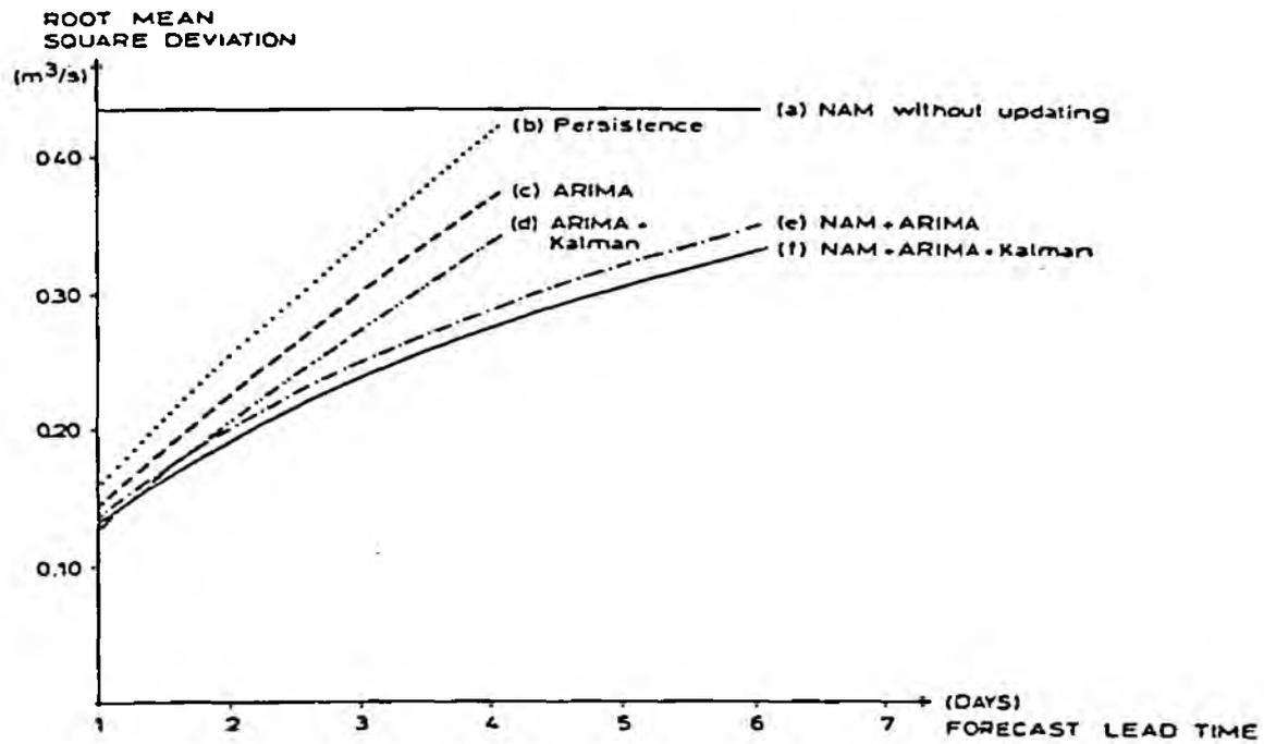
Figure 2.3 Forecasting error as a function of lead time from Refsgaard and Havnø, 1981.
