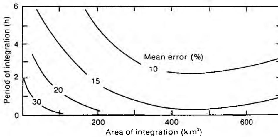
Mean error (without regard to sign) in the measurement of areal rainfall using a radar calibrated against a single raingauge, plotted as a function of the area and period of integration. (From Collier 1977.)
