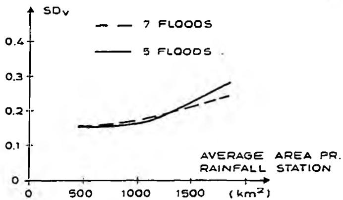
Figure 3.4 Discharge forecast accuracy as a function of raingauge network density, from DHI/CWC, 1983.
