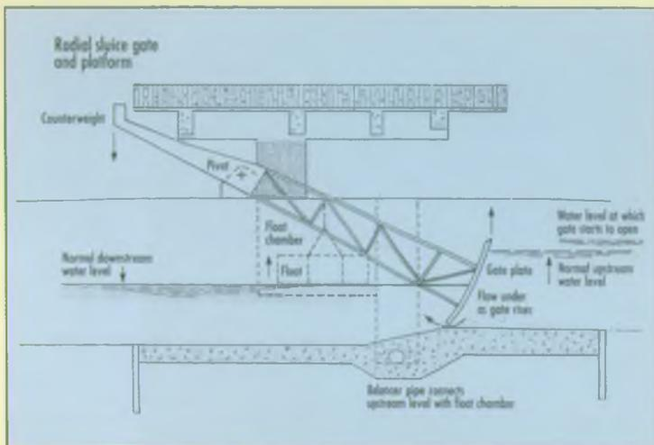
*The radial gate opens automatically as levels rise upstream. A pipe connects to float chambers either side of the gate. As the levels rise, so large hollow metal boxes connected to the gate float up overcoming the counterweight. This raises the gate plate, allowing more water to flow through*
