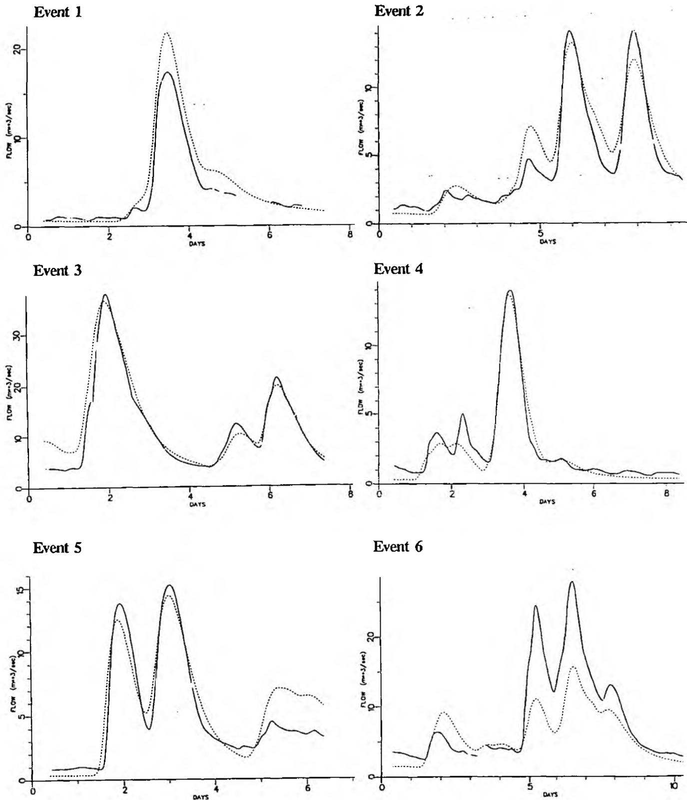
**Figure 6.5.1** Calibration results for the Thames Conceptual Model of the River Mole at Kinnersley Manor. Solid lines show observed flow, dashed lines show simulated flow.
