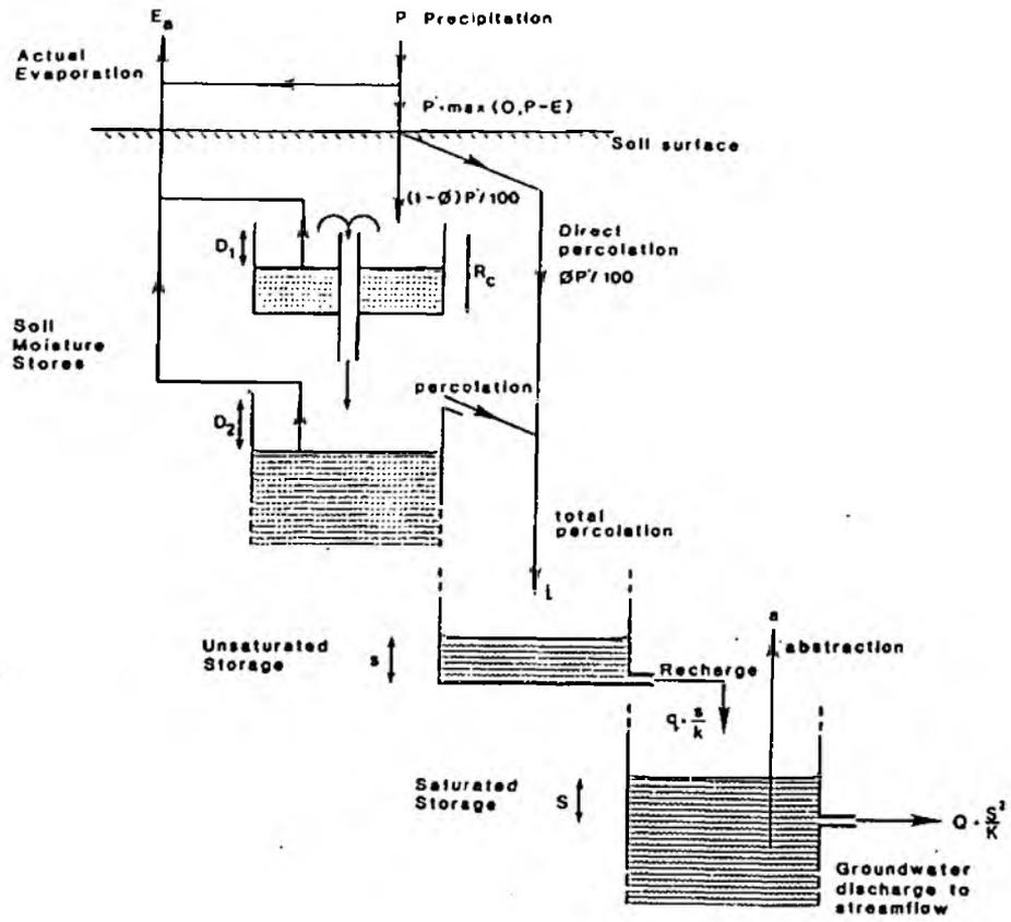
Figure 3.2.1 Representation of a hydrological response zone within the Thames Conceptual Model
