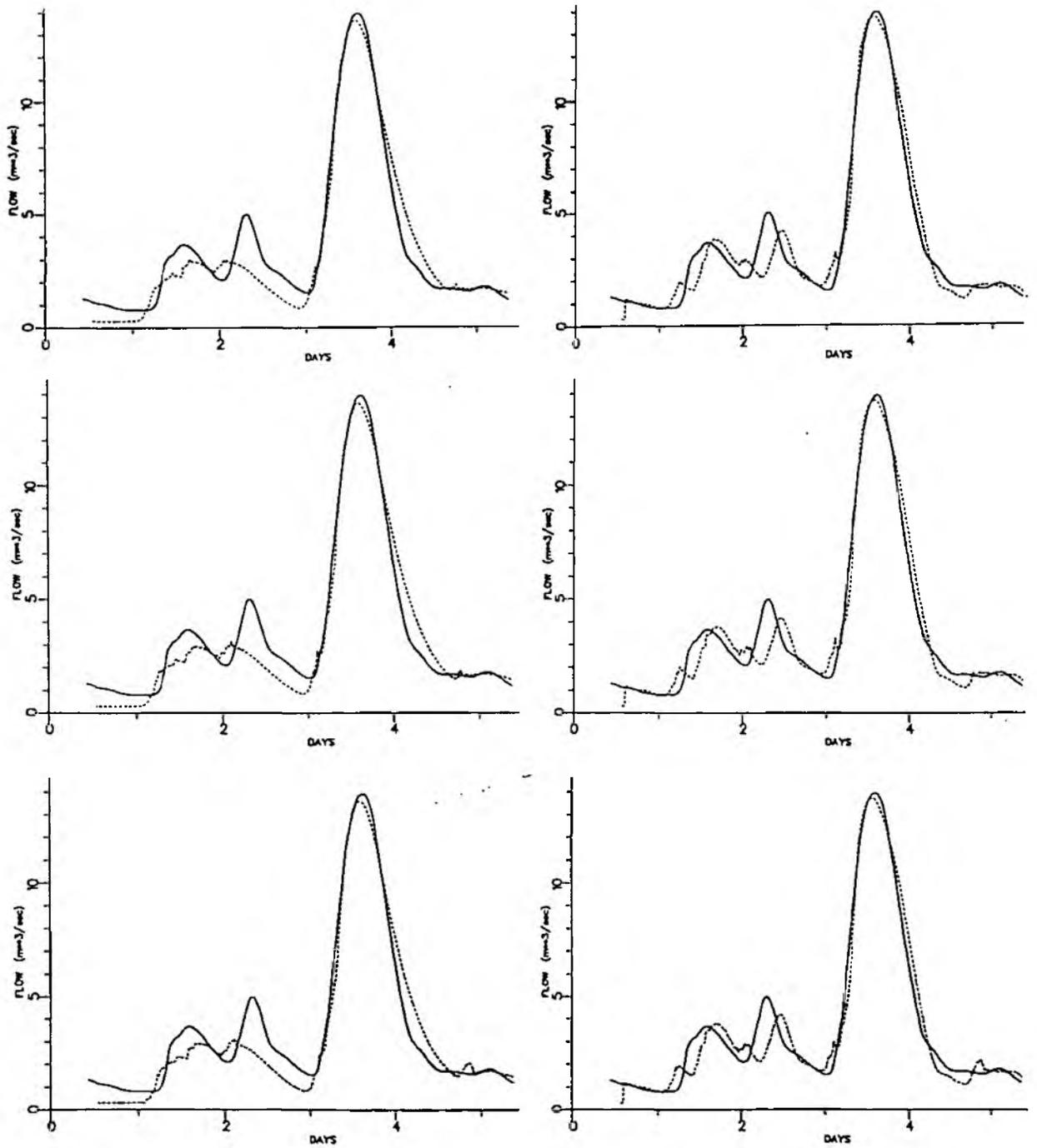
**Figure 6.5.3** 4-hour fixed lead-time forecasts for the event of 25-30 October 1990. Thames Conceptual Model of the River Mole at Kinnersley Manor. Solid lines are observed flow, dashed lines are forecasts. Results for simulation mode (left) and error-prediction mode (right) using forecast rainfall given by observed radar (top), local forecast (middle) or FRONTIERS forecast (bottom).
