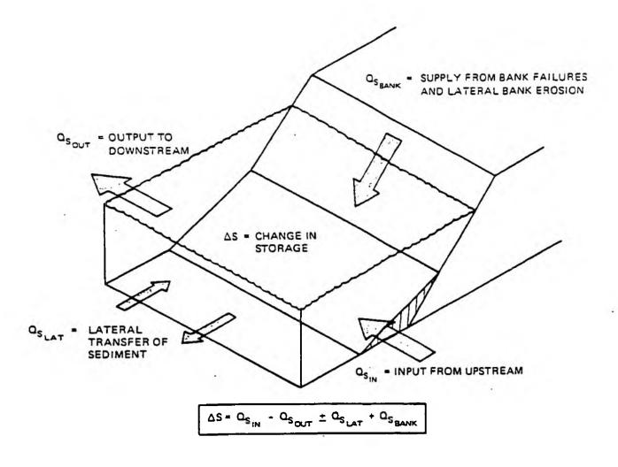
Figure 1. Sediment Movement into and out of the near bank zone. The sediment balance determines the rate of toe scour or spending beach accumulation at the foot of the bank and this ultimately determines the rate of bank retreat.
