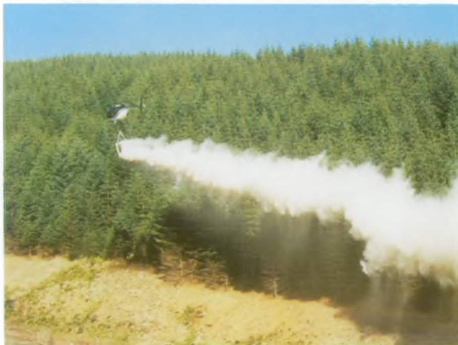
Liming operation to reduce effects of acidification on upland stream (Welsh Region)
