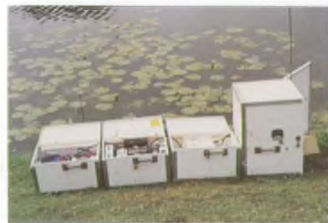
Sberlock automatic water quality monitoring device (Wessex Region)
