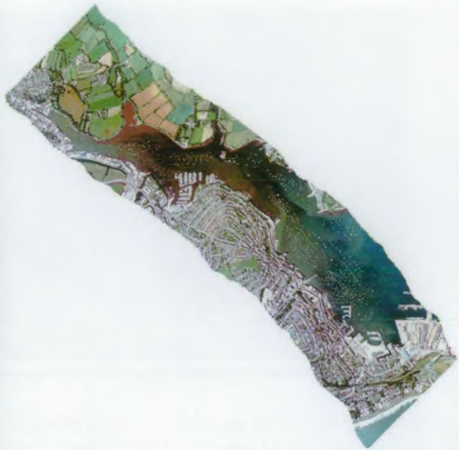
Figure 5. CASI true colour composite showing the presence of red algae in the Fal Estuary
