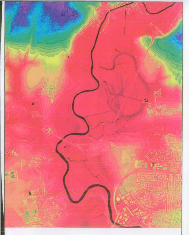
Digital elevation model (DEM) of the River Arun catchment created from LIDAR data flown on the 22/7/97
