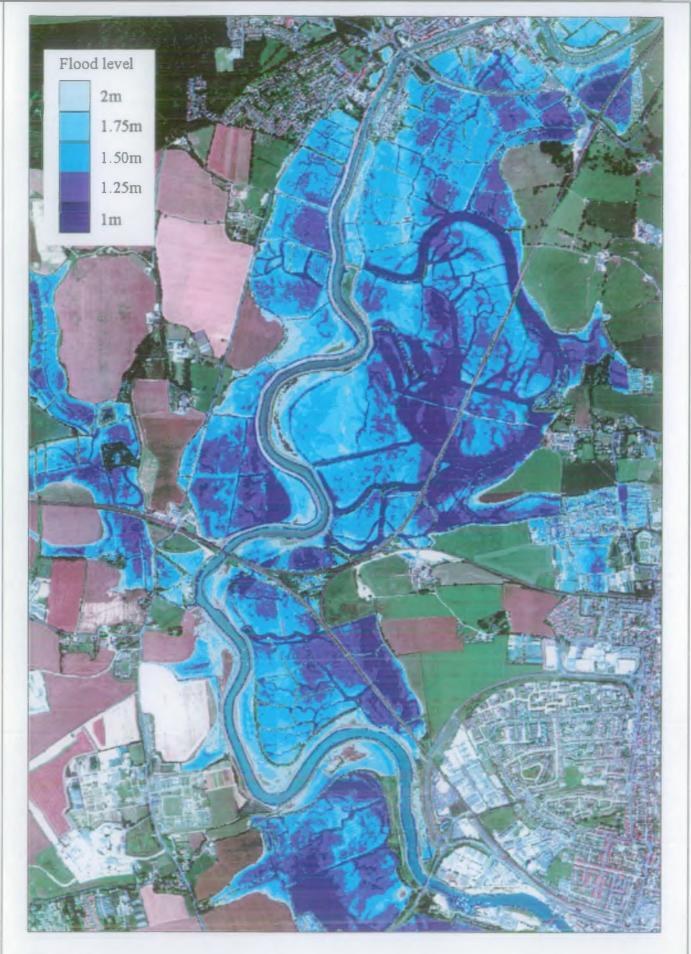
Plate 6 CASI true colour composite overlaid with areas affected by 20cm increases in flood level between 1m and 2m
