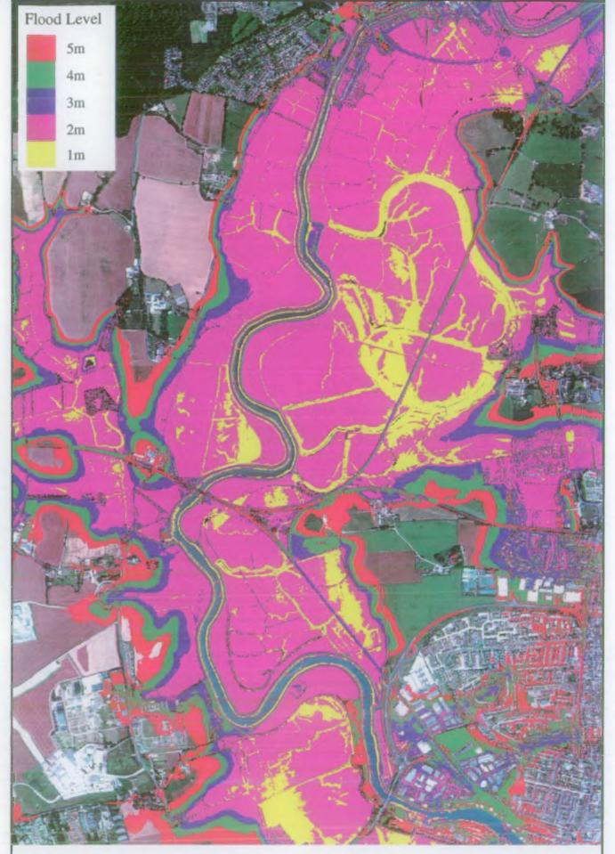
Plate 5 CASI true colour composite overlaid with areas affected by different levels of flood
