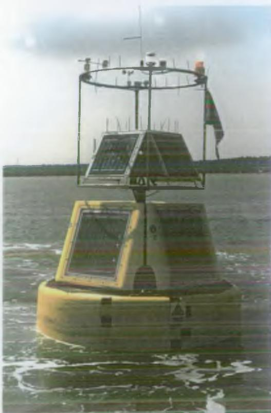
5.2 The Proteus buoy holds sensors for temperature, salinity, dissolved oxygen, pH, fluorescence, transmission and nitrate. Further developments are being made to integrate sensors for additional nutrients. In order to investigate the fate of OSPAR monitored hazardous substances it would be necessary to collect water samples for analysis onshore. The current telemetry system allows for both
