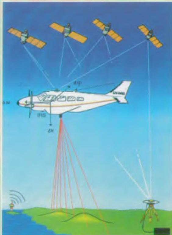
LIDAR system: Operational links
