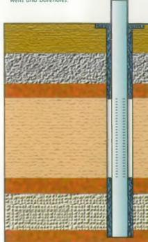
in Section 4 (above) indicates that the boreholes intersect important aquifer units (in terms of resource and quality), and are constructed so that representative groundwater samples may be collected or water levels measured. The ideal borehole construction and completion is dictated by the geological strata encountered and its intended use. Boreholes which intersect a single aquifer unit may be cased through the unsaturated zone, but open hole
