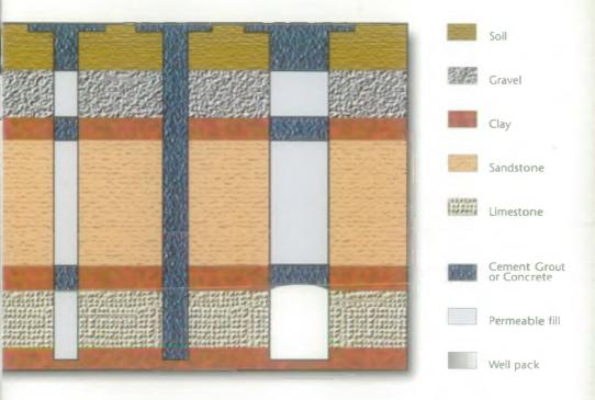
(or screened) below the watertable. Boreholes in more complex geologies are likely to require casing over most of the depth of borehole with the exception of the aquifer unit(s) of interest (*see Fig.2 (A*)). These details must be established when considering conversion of the borehole to a monitoring point along with the ultimate purpose that the monitoring facility will serve.
