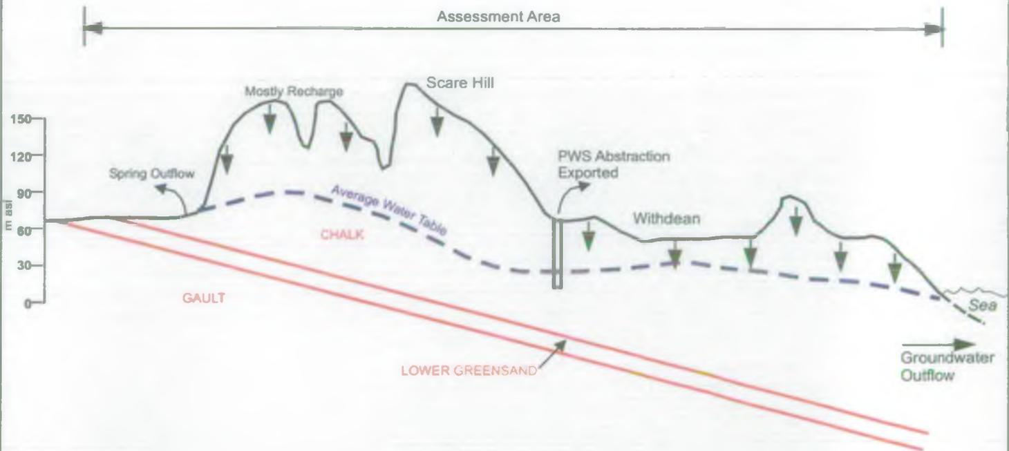
**FIGURE 9.3 BRIGHTON CHALK BLOCK: CONCEPTUAL SKETCH PLAN AND SECTIONS**
