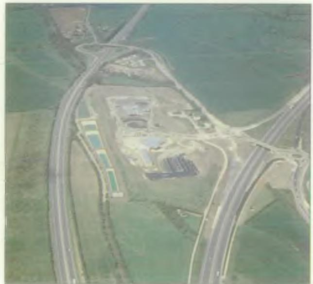
*Sustainable Urban Drainage techniques were incorporated into this new roadside service area on the M40 from the earliest planning and design stage. SUDS provided the most economic means of protecting the local watercourse from flooding and pollution.*
