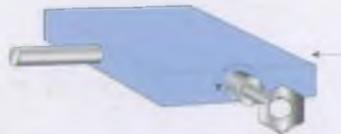
When the gate is either fully raised or lowered, re-lock the winding gear by relocating the slide bolt, while holding the slidebolt with the thumb, push in and relock the abloy lock barrel. Remove the key
