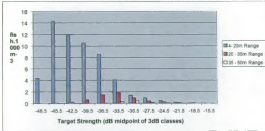
**Figure 7: Mean volume density by acoustic size class for 3 ranges from the transducer – Combermere.**
