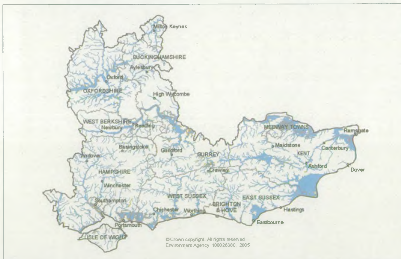
Figure 10: Flood risk areas make up 11 per cent of the total land area in the South East. More than 235,000 properties and £50 billion worth of assets are at risk of flooding in the region. Much of the flood risk area is defended, reducing the residual risk to development in this area.
