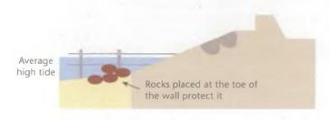
Figure 4 Use a rock toe to protect the wall, option 4
