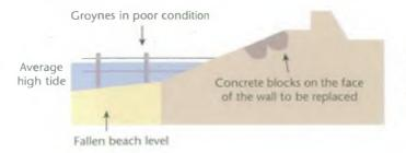
Figure 2 Current condition of the flood defences, option 2
