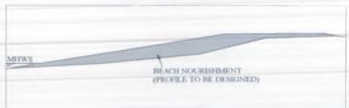
Cross-section of typical beach nourishment defence
