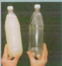
Bottles of creamery effluent before and after treatment
