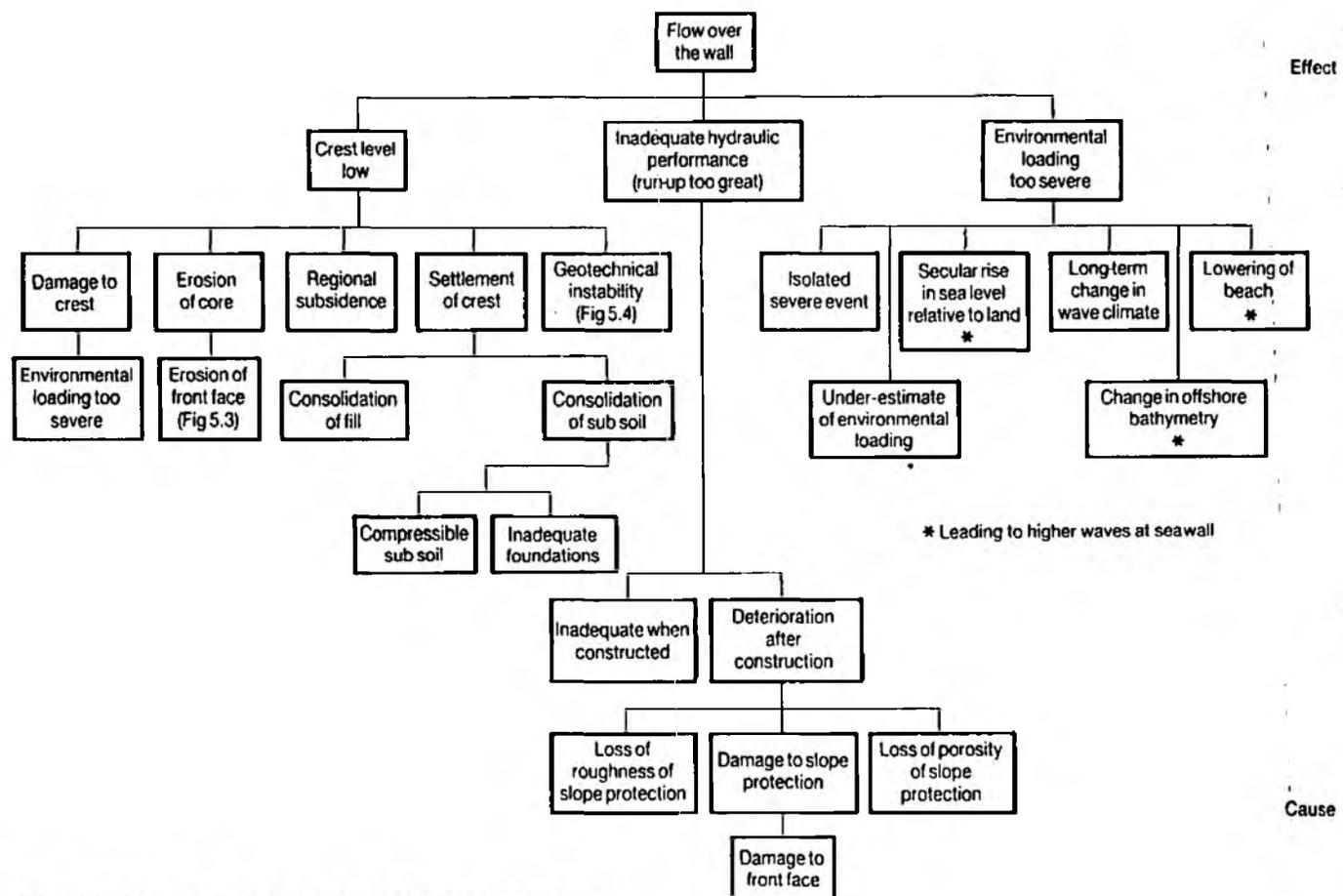
Figure 5.2 Fault tree: Events leading to flow over seawall
