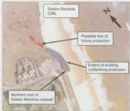
Possible outflanking protection works at Easton Marshes
