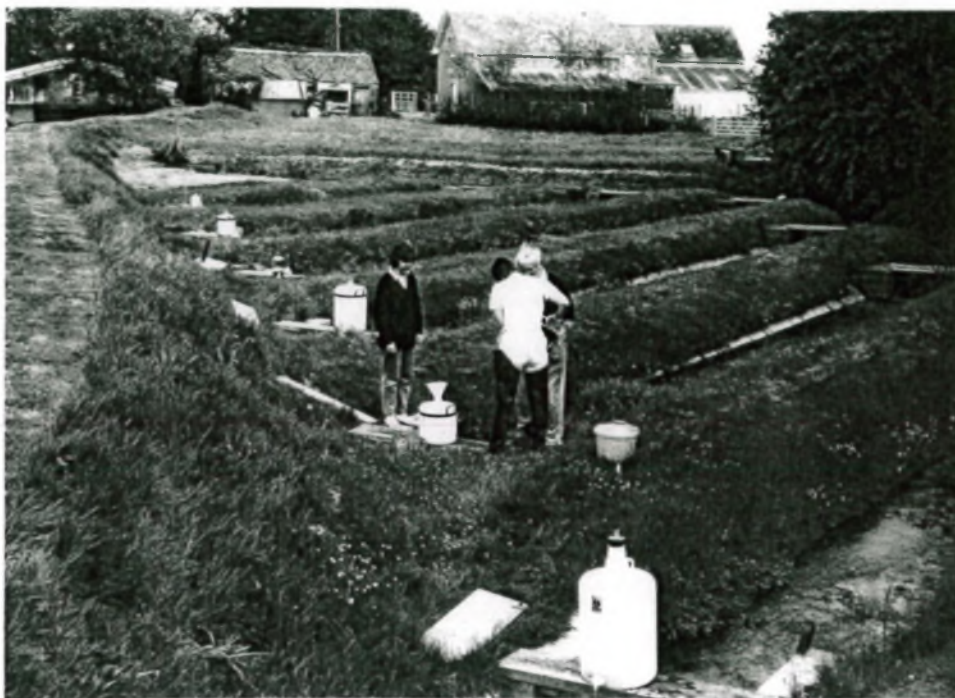
Plate 2. View of the channels showing the drip feeds in position
