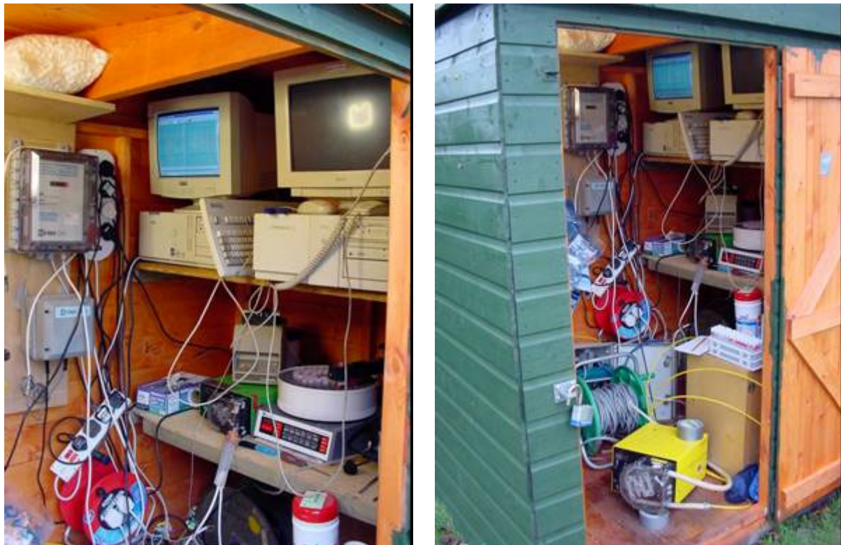
Figure 4.4 Field laboratory set-up for field tracer tests
