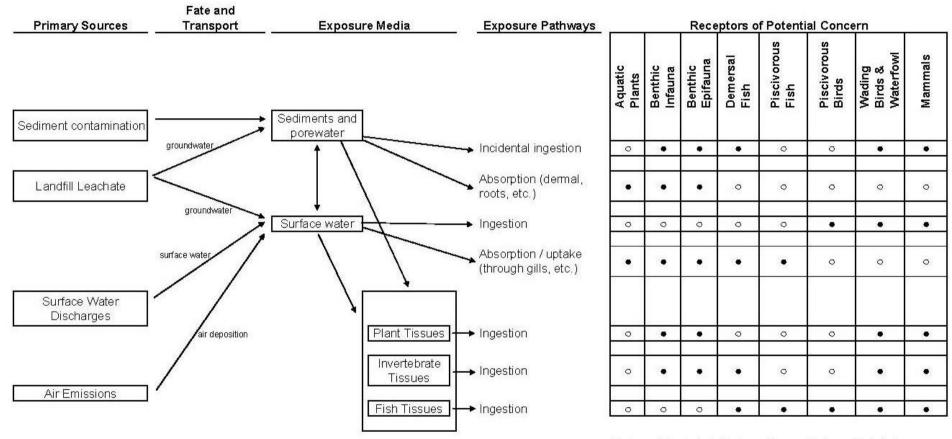
Figure 3.5 Box diagram CSM – example 1
