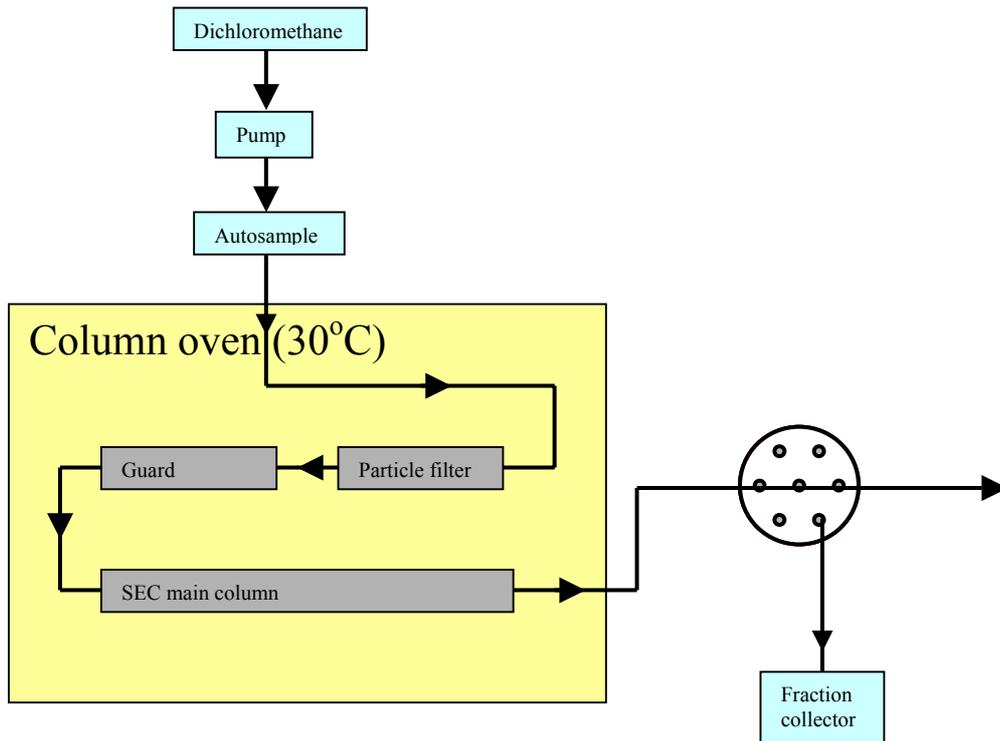
Figure 9.3. Schematic of the HPLC system for the fractionation of PAHs and PCBs
