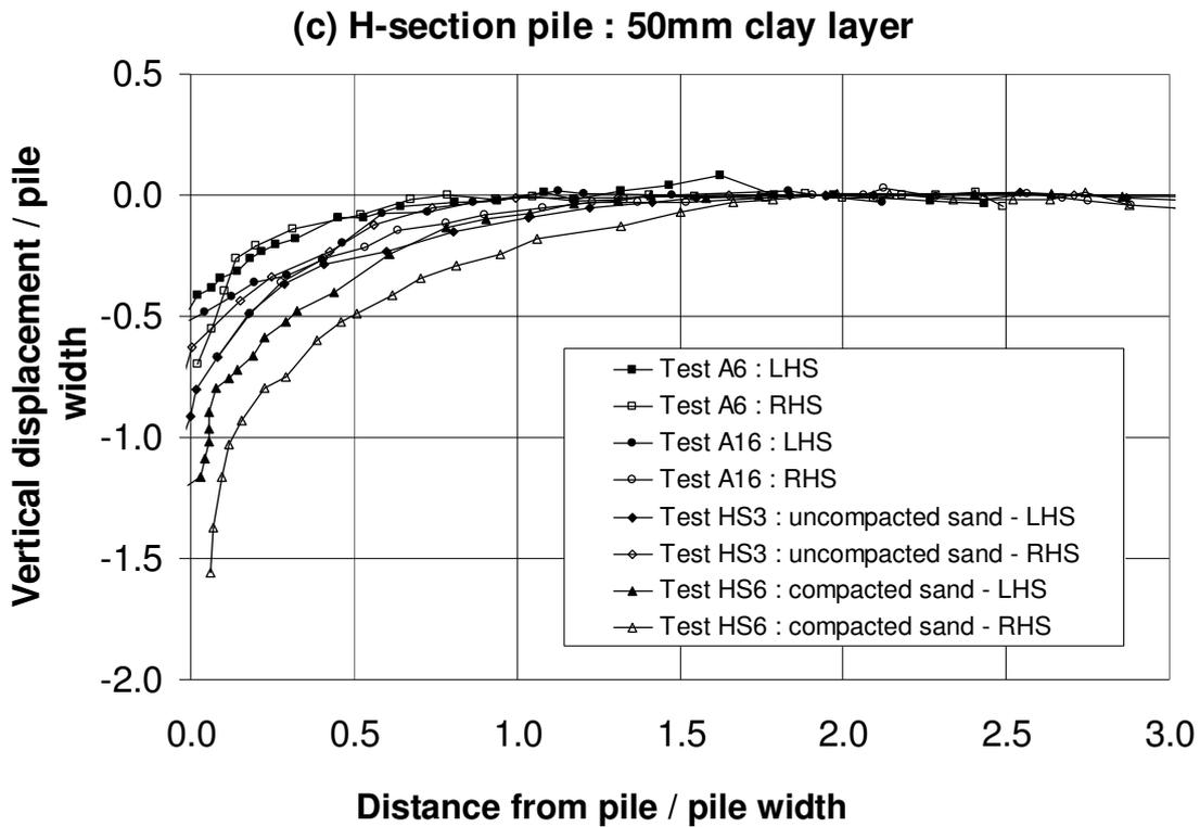
**Figure 4.13. Comparison of axisymmetric and half-section test results for vertical displacement**
