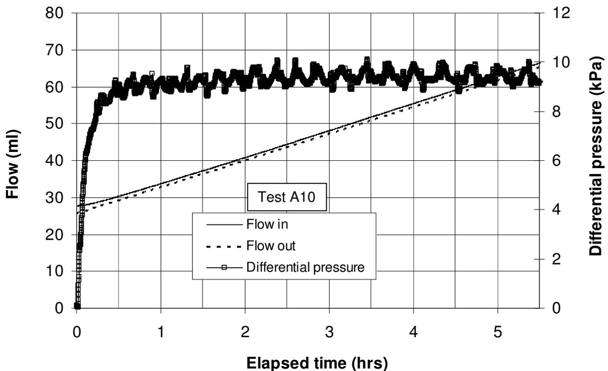
Figure 4.16. Example of GDS flow pump test result before model pile construction
