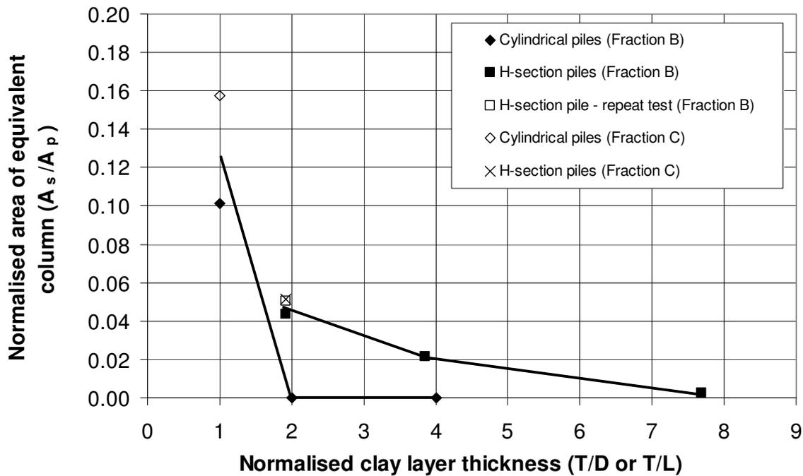
**Figure 4.19. Normalised plot of equivalent column area versus clay layer thickness**
