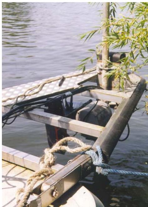
Figure 2.5. Transducer mounting on *Pingu*. The transducers and rotator were submerged once alignment had been checked
