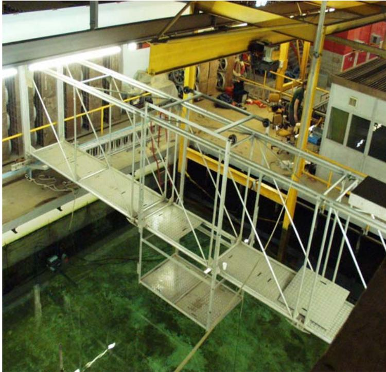
Figure 2.2. Gantry over tank used for suspending targets
