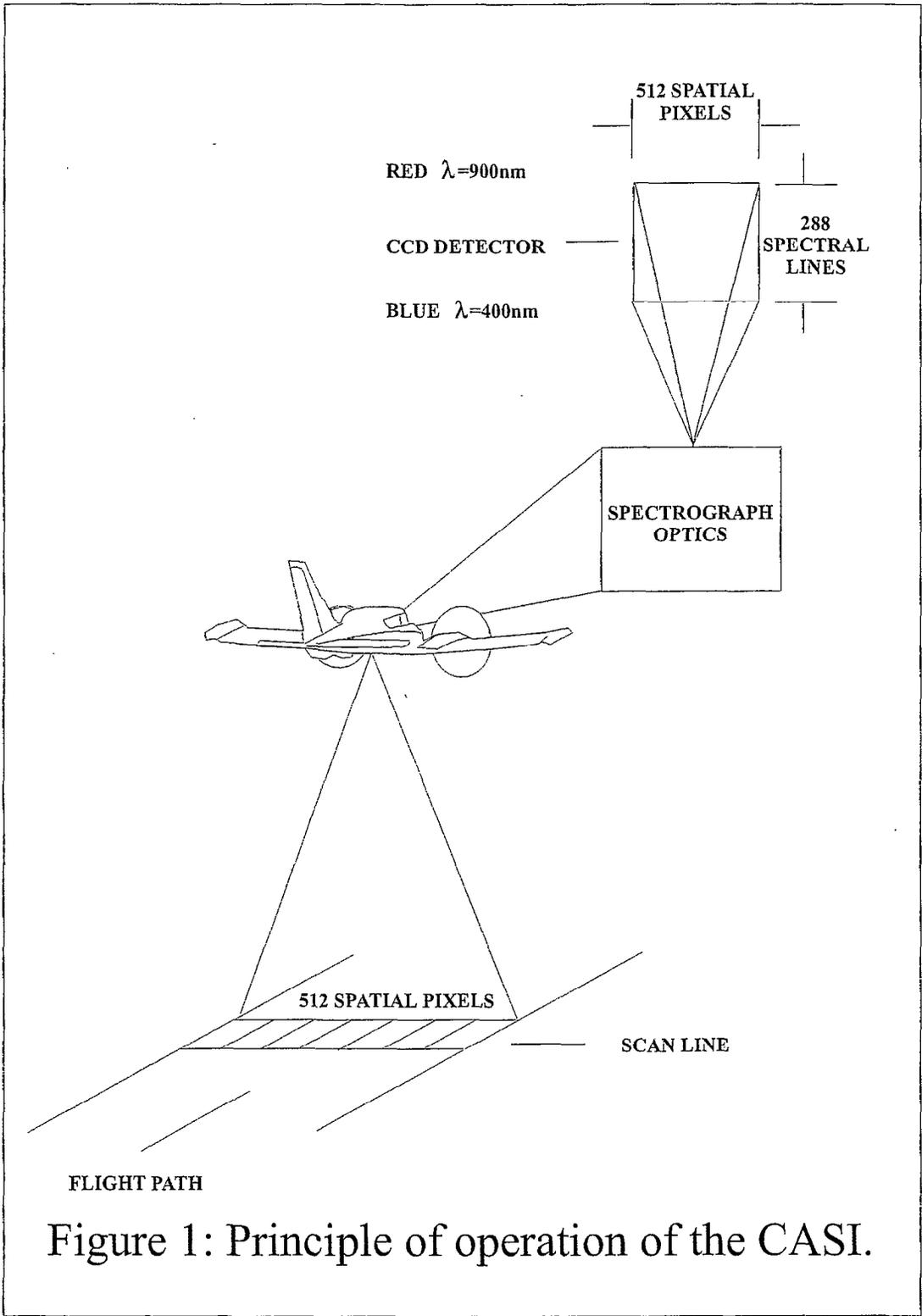
Figure 1: Principle of operation of the CASI.
