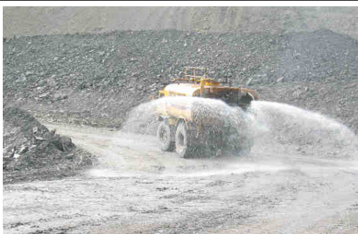
Photo A9.21 Dust suppression on haul roads by bowser
