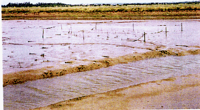
Figure 2.8 Remains of Tollesbury planting experiments that failed due to the low elevation (Section 2.3.1).
