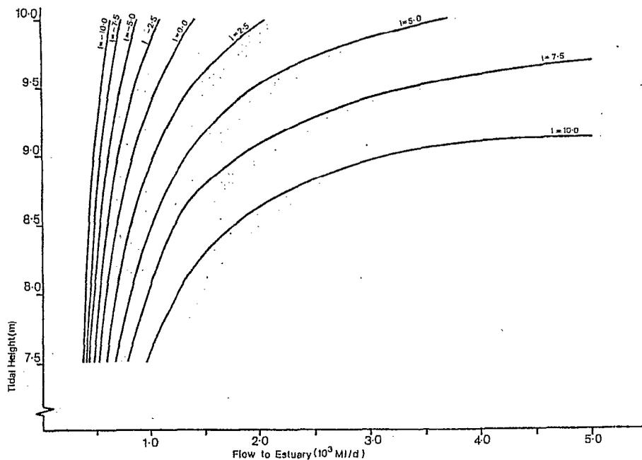
**Figure 13.7 - INTRUSION FOR COMBINATIONS OF FLOW AND TIDE**
