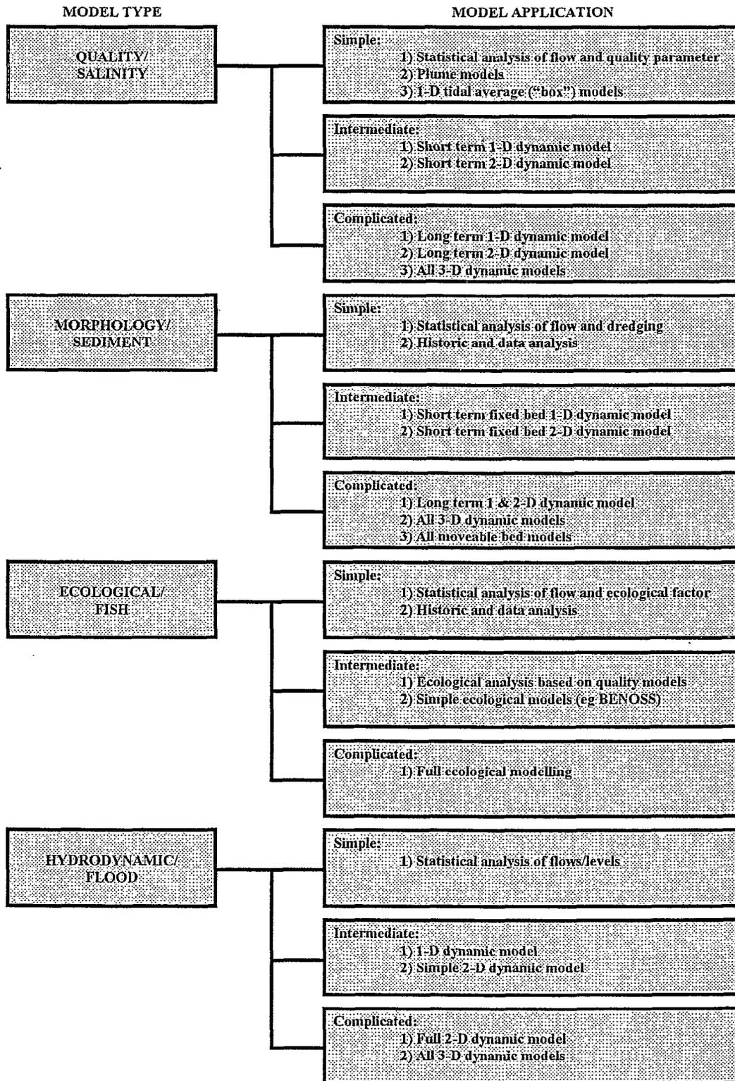
Figure 8.9 - COMPUTATIONAL MODEL APPLICATIONS
