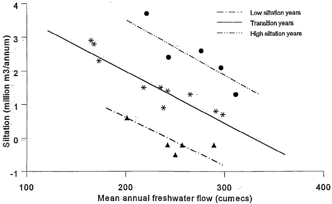
Figure 1.1 - SUNK DREDGED CHANNEL - RELATIONSHIP BETWEEN MEAN ANNUAL FRESHWATER FLOW AND ANNUAL SILTATION
