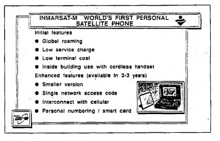
Inmarsat-M's all-digital telephony at 4.8 kbit/sec and 2.4 kbit/sec data and facsimile services will appeal to both maritime and land customers in applications where voice communications, a high degree of portability and lower cost are important.
