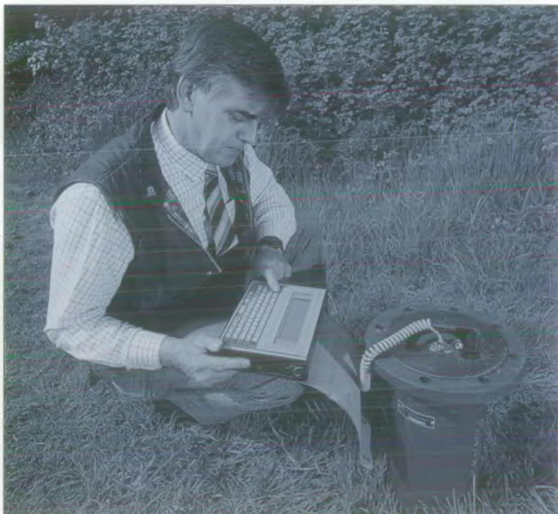
Collecting groundwater level and quality information from a datalogger
