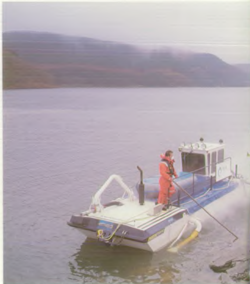
The NRA is fighting acid rain in Mid Wales with a new Swedish-built boat used to lime the waters of Llyn Brianne. The main aim is to have a beneficial impact on river quality in the important River Tywi fishery downstream.
