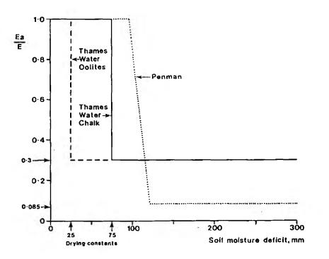
Figure 3.2.2 Representation of actual evaporation, E, as a function of potential evaporation, E, and soil moisture deficit
