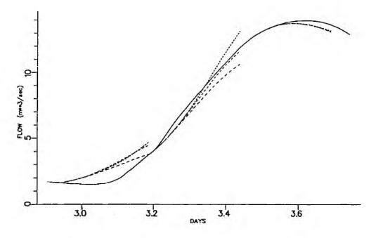
Figure 6.5.2 Fixed-origin forecasts at 16, 10 and 4 hours before the main hydrograph peak for the event of 25-30 October 1990. Thames Conceptual Model of the River Mole at Kinnersley Manor. Forecasts made using observed radar data (short dashes), local radar rainfall forecasts (medium dashes) and Frontiers forecasts (long dashes) as input. Solid lines are used for the observed flow.
