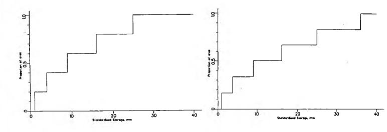
Figure 3.5.2 Runoff production component of the SUHM model: distribution functions of storage capacity, in standardised form, used for paved and riparian areas
