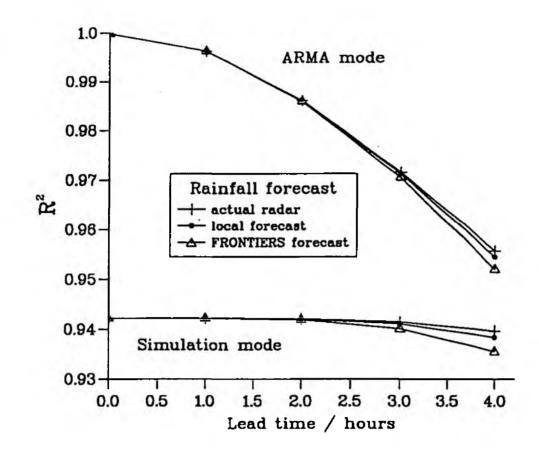
Figure 6.5.4 Forecast performance with increasing lead time for the Thames Conceptual Model of the River Mole at Kinnersley Manor during the event of 25-30 October 1990.
